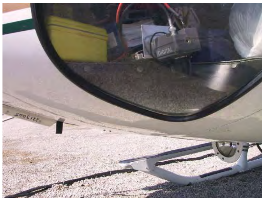
Figure 6. Digital video camera typical mounting location
