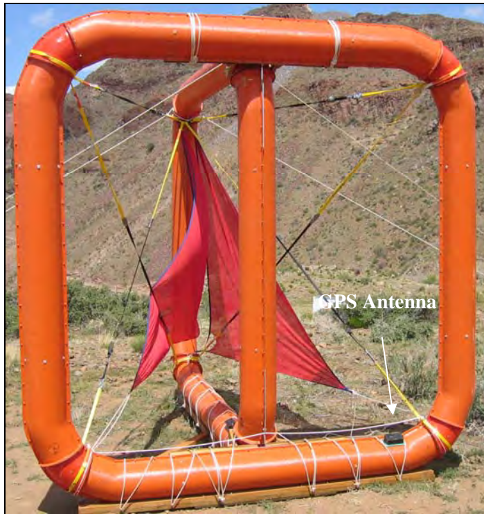
Figure 5 - ZTEM base station receiver coils.
