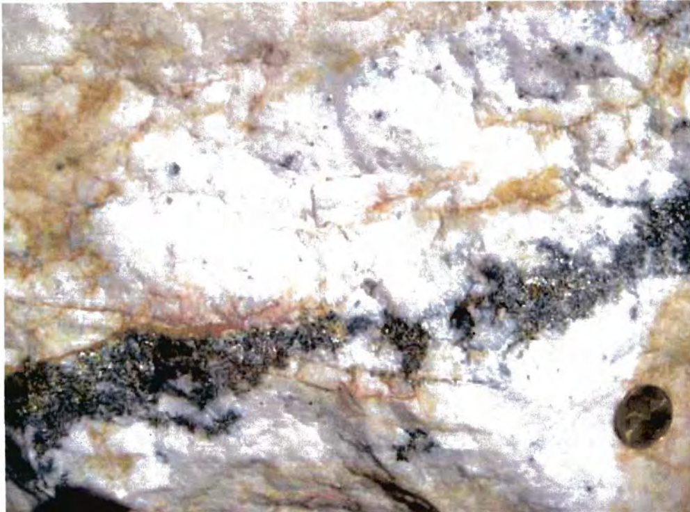
Photo 2. Sulphide mineralization including chalcopyrite, pyrite and galena in the main vein trench. Location NAD 83, Zone 17, 494339E, 5306416N.
