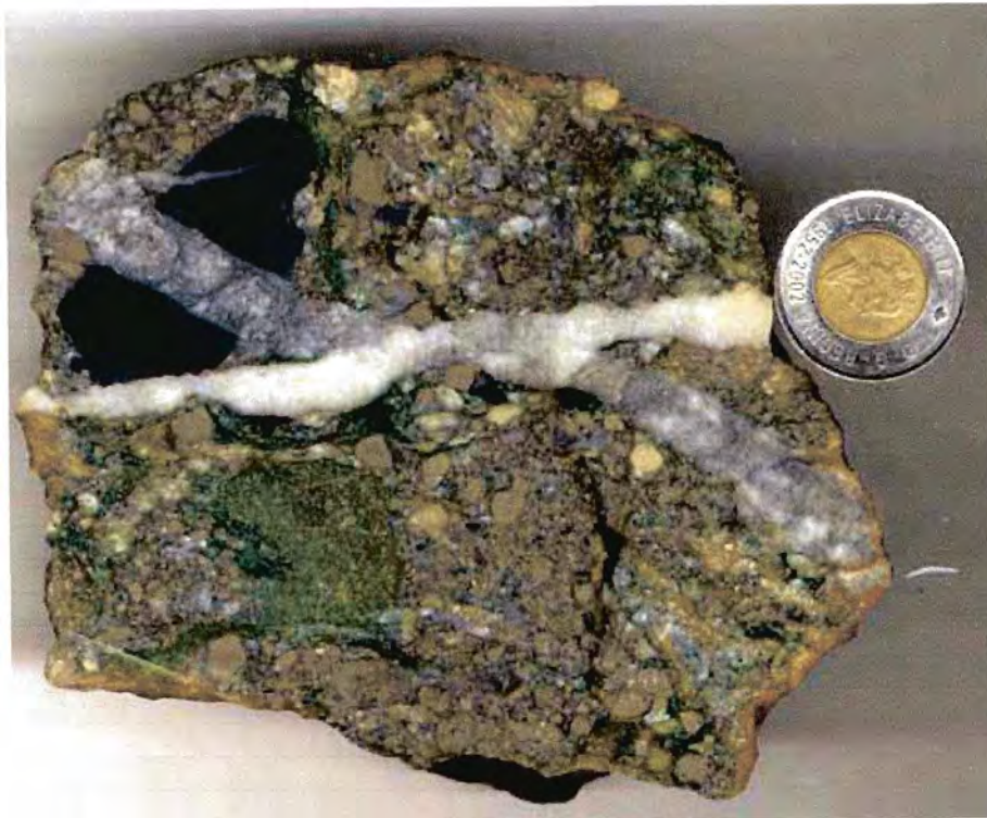
Photo 6. Timiskaming clast supported conglomerate from the Midlothian Township Sylvanite Gold Mines Ltd. Occurrence. A black argillite clast is cross-cut by iron carbonate veinlet which is subsequently offset and cut by a late quartz vein. Several generations of fine to coarse grained pyrite are evident in the rock sample as are a variety of clast types including fuchsite clasts, felsic volcanic and lithic clasts. Location, UTM NAD 83 Zone 17, 494915E, 5306384N.
