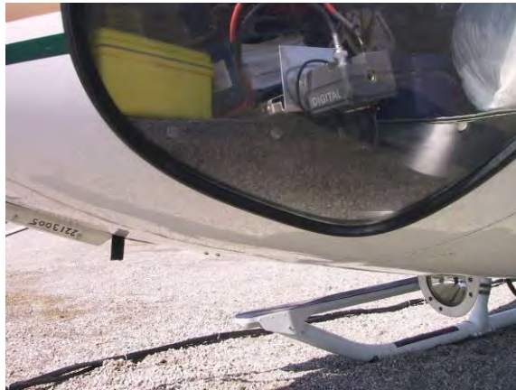
Figure 6. Digital video camera typical mounting location
