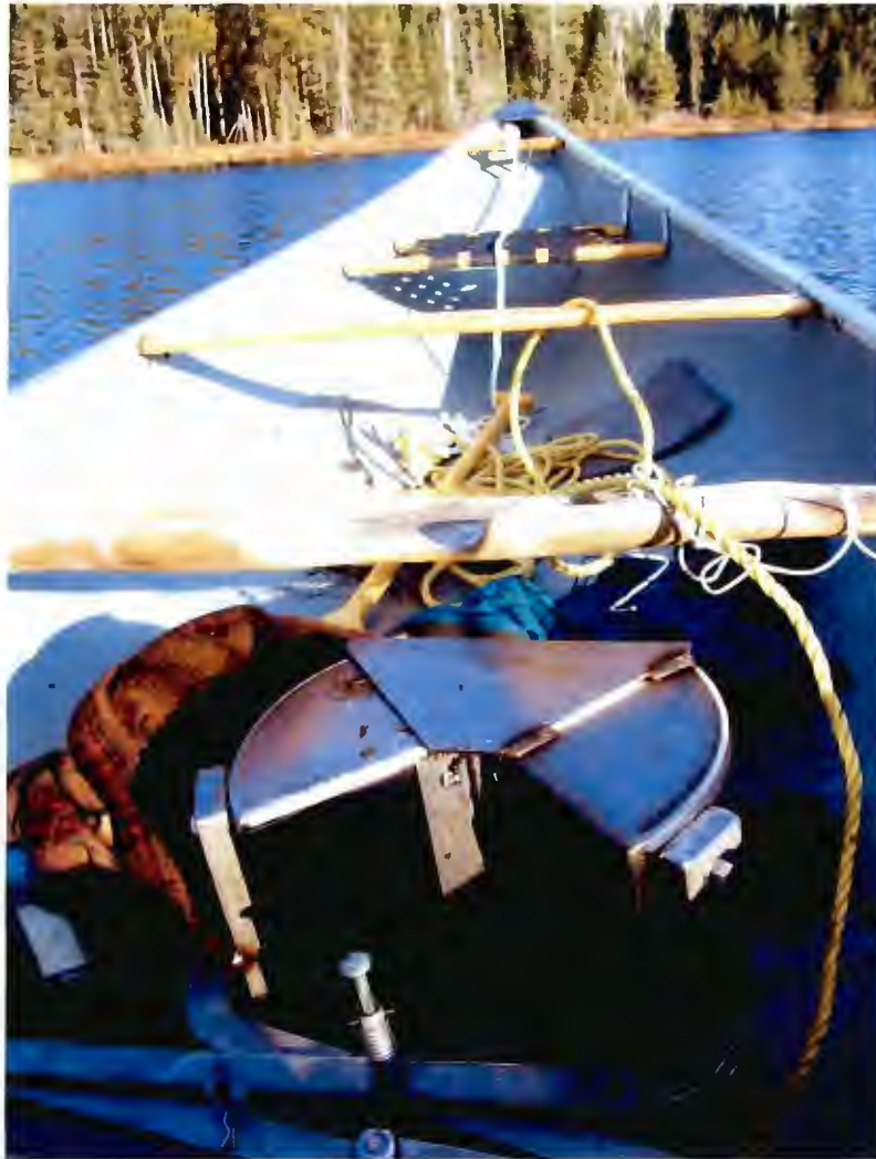
Clam-shell sampler used to collect lake-bottom SGH samples
