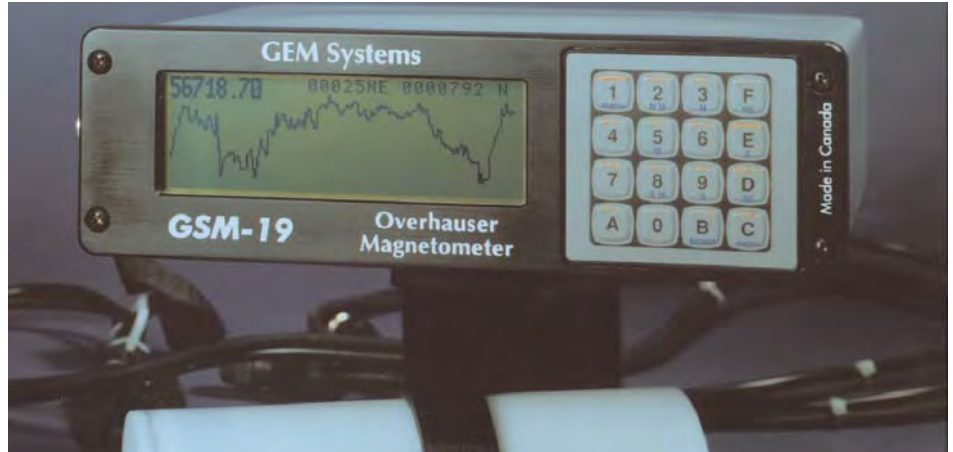
Overhauser (GSM-19) console with sensor and cable. Can also be configured with additional sensor for gradiometer (simultaneous) readings.
