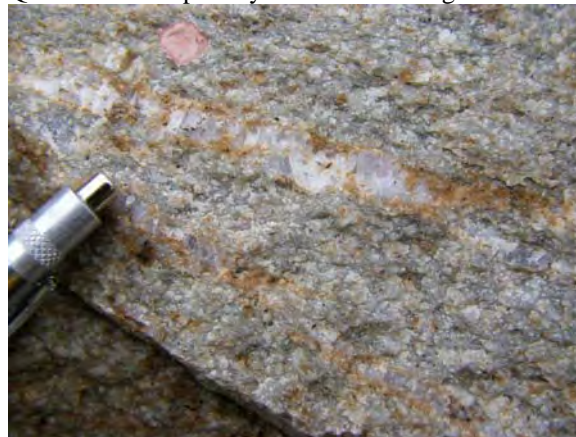
Quartz ± sulphide veinlets in sericitized porphyry. Gold: 301 ppb
