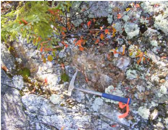
Quartz vein with selvages up to 3% fine pyrite
