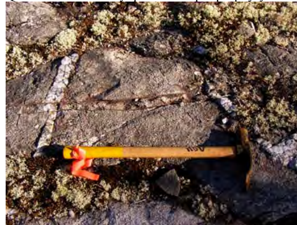
Poor-quality sawn-channel sampling
