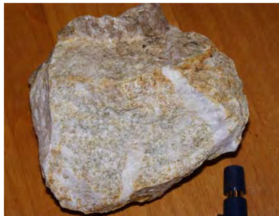
Sample 1204515: 19.81 ppm Au. Note intensive coarse sericite + patchy carbonate alteration
