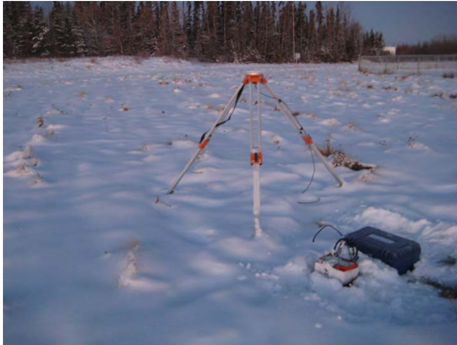
Figure 4. Typical GPS Base station setup
