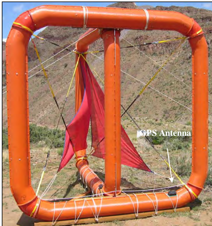
Figure 5 - ZTEM base station receiver coils.
