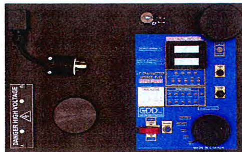
Face plate of the ←1800W and 3600W→ IP Tx
