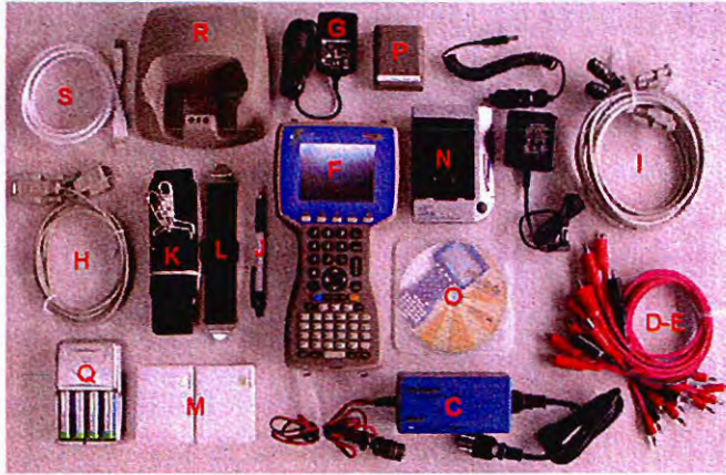
↕ Components included with GDD IP Receiver GRx8-32
