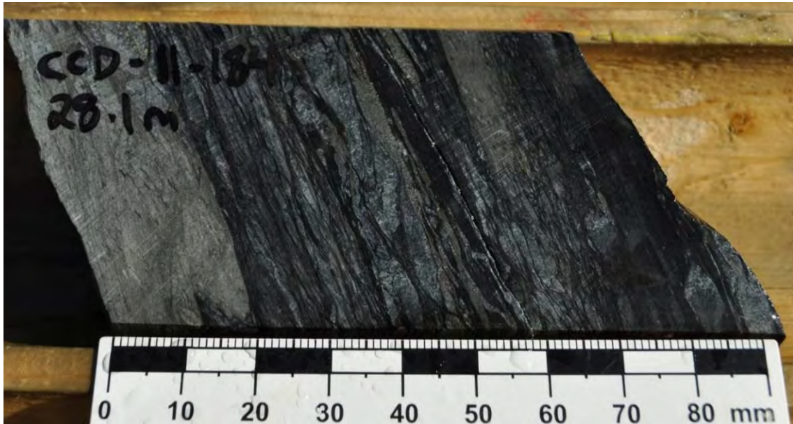
Figure 7: Carbonaceous sedimentary volcanoclastic rock with thin diagenetic pyrite lenses
