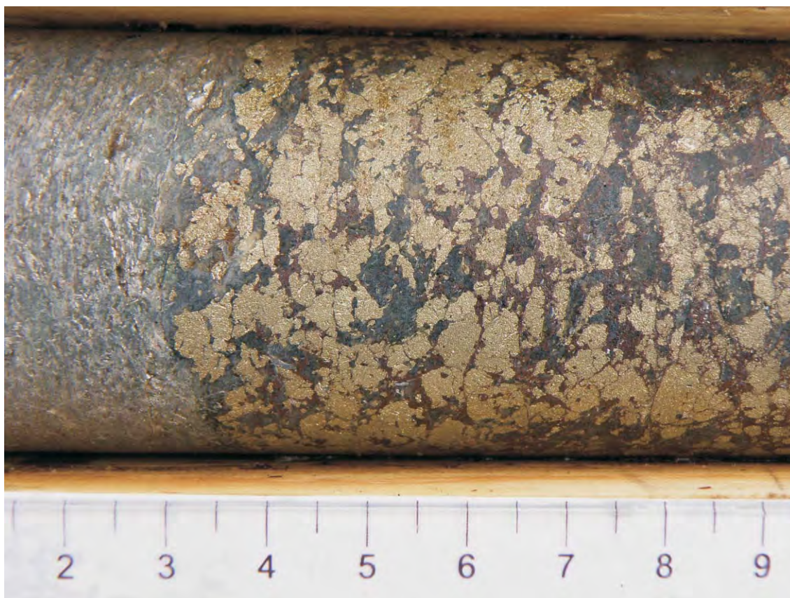
Figure 21. Gouda Lake zone drillcore from drillhole HEGZ10-19, showing the contact between pyritic white mica schist and massive pyrite-sphalerite-galena (trace); this section graded 0.245 g/t Au, 50.1 g/t Ag, 0.4% Pb, and 3.08% Zn over 1.5 m; Gouda Lake area, Hemlo East property.
