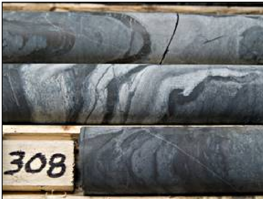
Figure 6 “E-Type” iron formation, magnetite-rich chert beds with interbedded magnetite beds. Note difference in magnetite content in F type chert above 308m.
