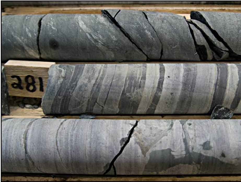
Figure 4 “F-Type” iron formation, lean chert beds with interbedded magnetite-rich chert beds and magnetite beds.
