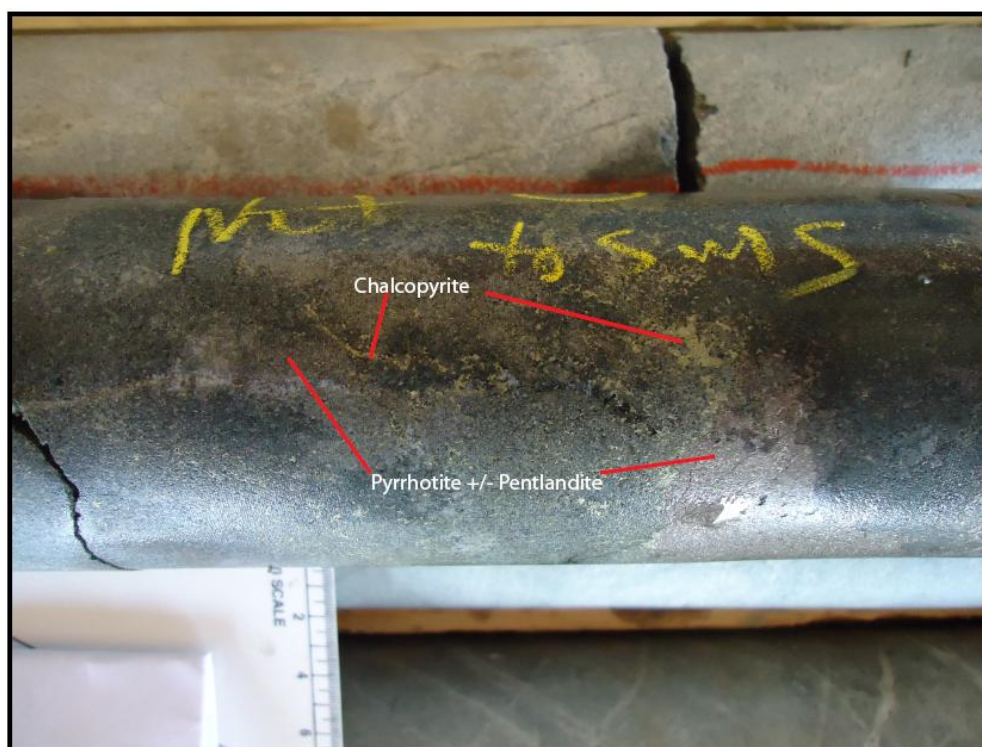
Figure 5: Net-textured to Semi-massive sulfide mineralization in drill hole NU-05-10, close-up of chalcopyrite and pyrrhotite +/- pentlandite.
