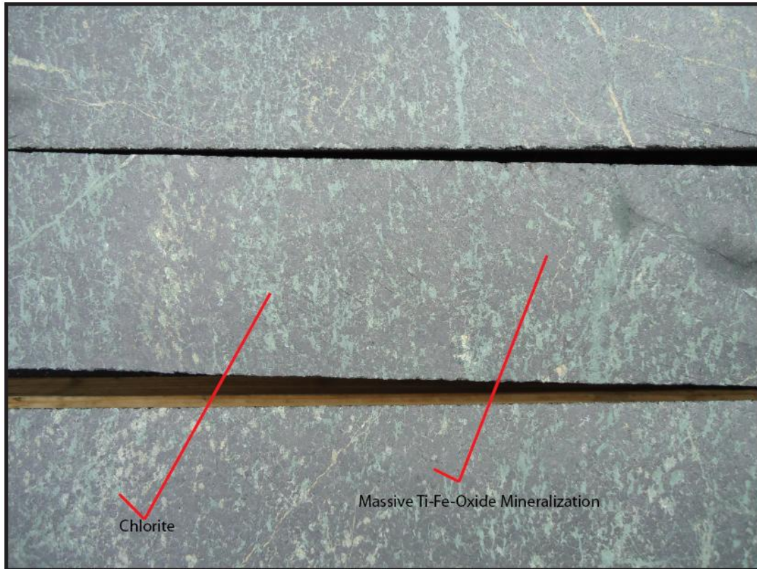
Figure 8: Massive titanium-iron-oxide mineralization in drill hole NU-06-10 with interstitial chlorite alteration, indicating a likely hosting parent rock of pyroxenite.
