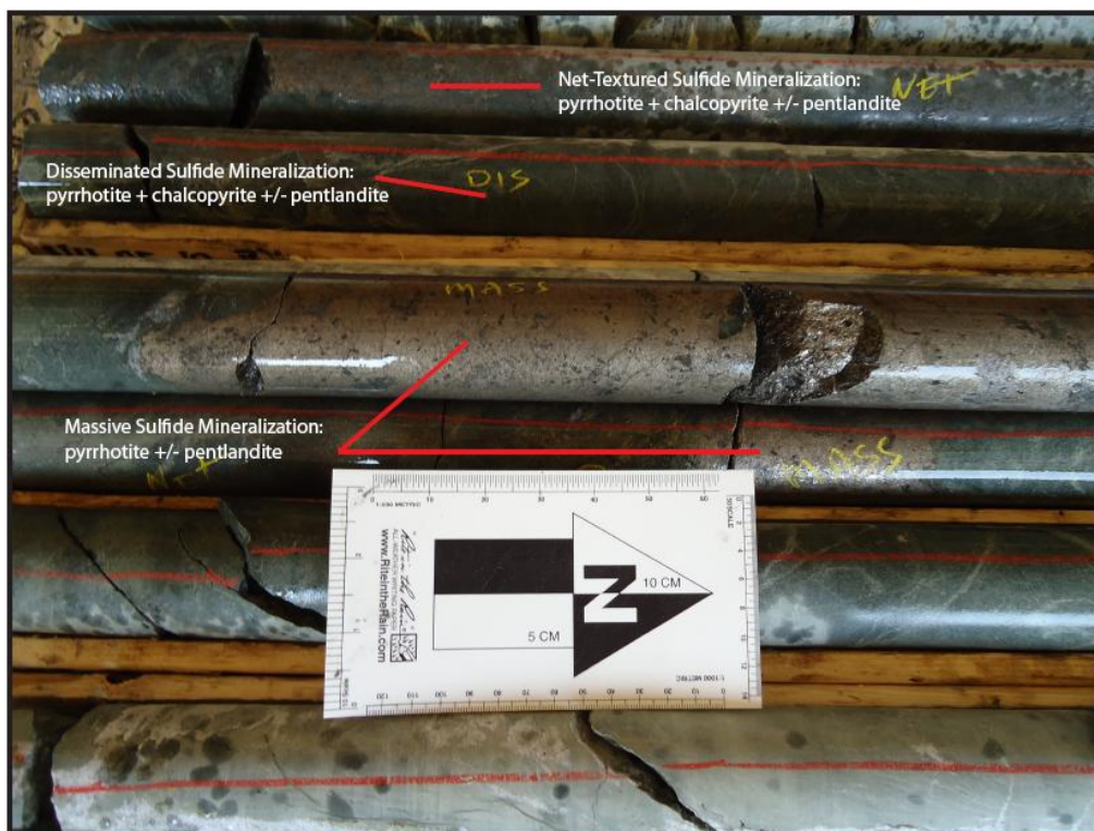
Figure 4: Photograph of massive, net-textured, and disseminated sulfide mineralization in drill hole NU-05-10.
