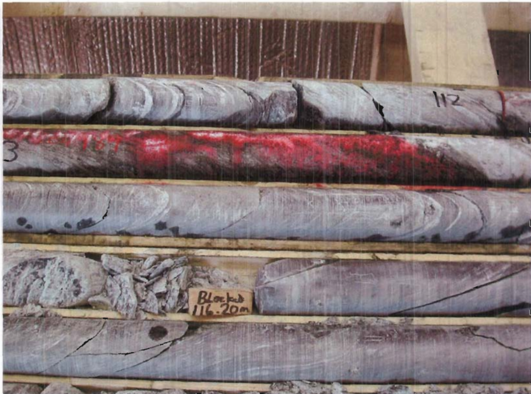
DSCN 2141. Pentlandite in 0407-119 at 113m. This is typical type 1A/2A mineralisation.
