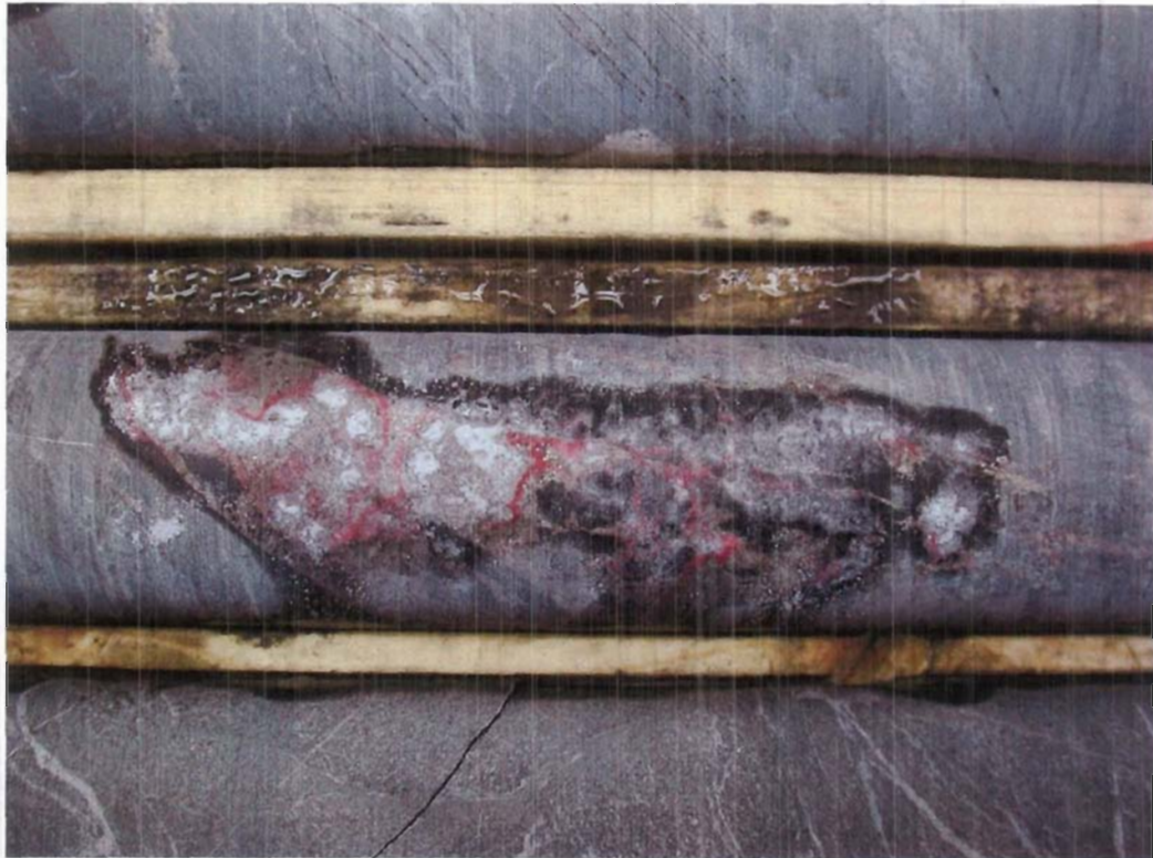
DSCN 2152. Coarse clusters of sulphides in MZ2AF1. Pentlandite and pyrrhotite picked out by nickel-zap accelerated with HCl.
