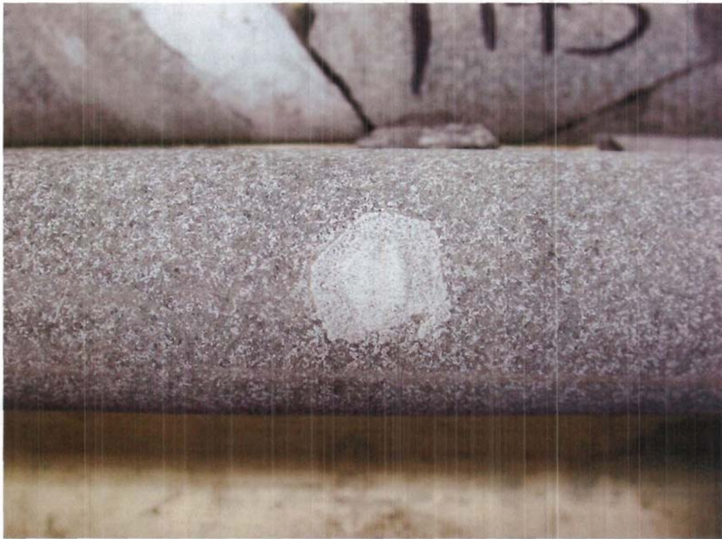
DSCN 2090. Relict partially digested zoned feldspar in 9D.
