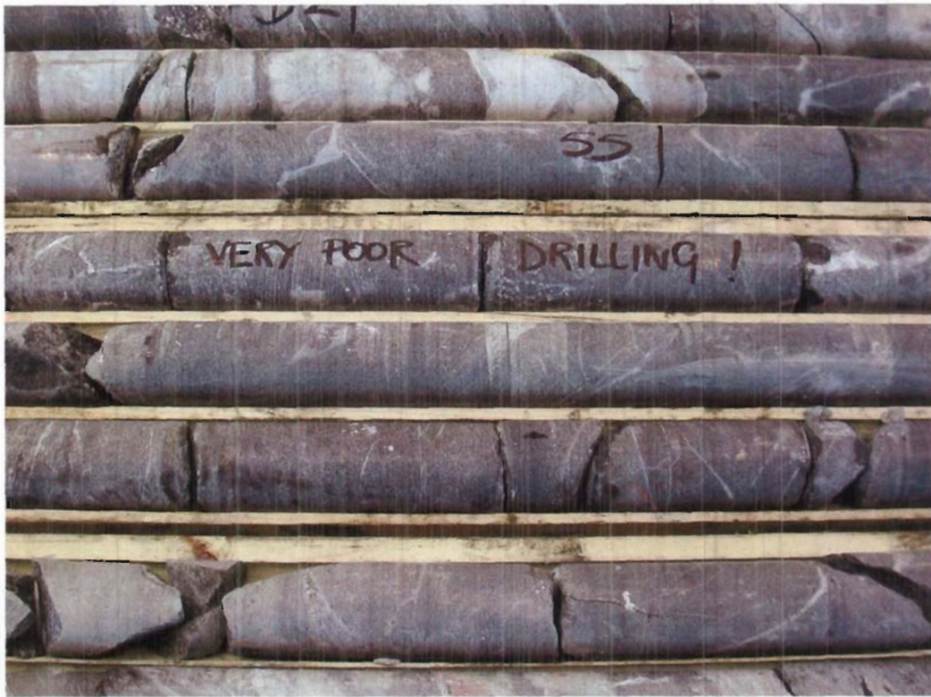
DSCN 2034. Core lost by grinding due to inexperienced drillers.
