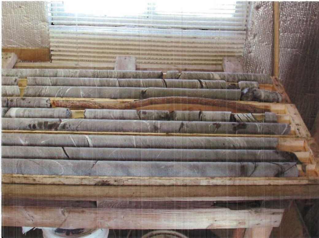
DSCN2020. Quaint practices to denote lost core. This is not really the done thing in diamond drilling. Two core blocks would suffice.
