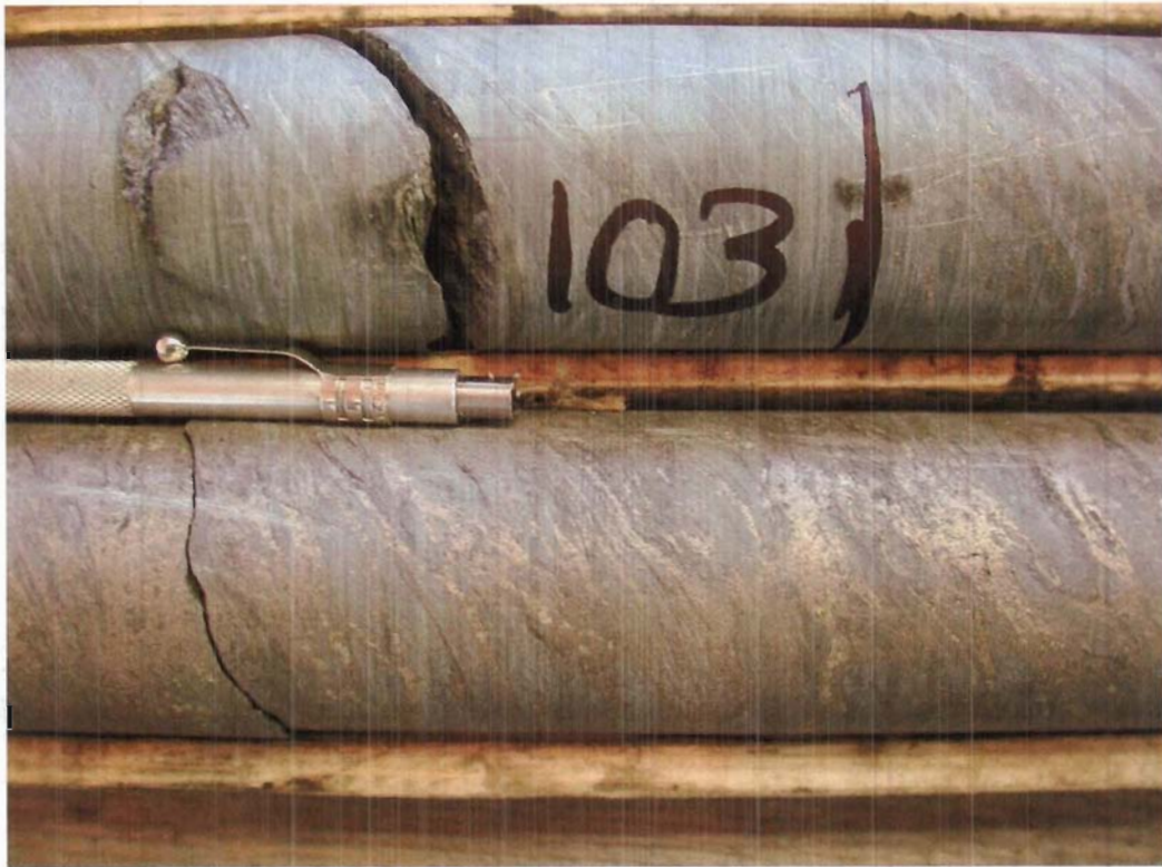
DSCN 2042. MZ2A with pyrrhotite and minor chalcopyrite.
