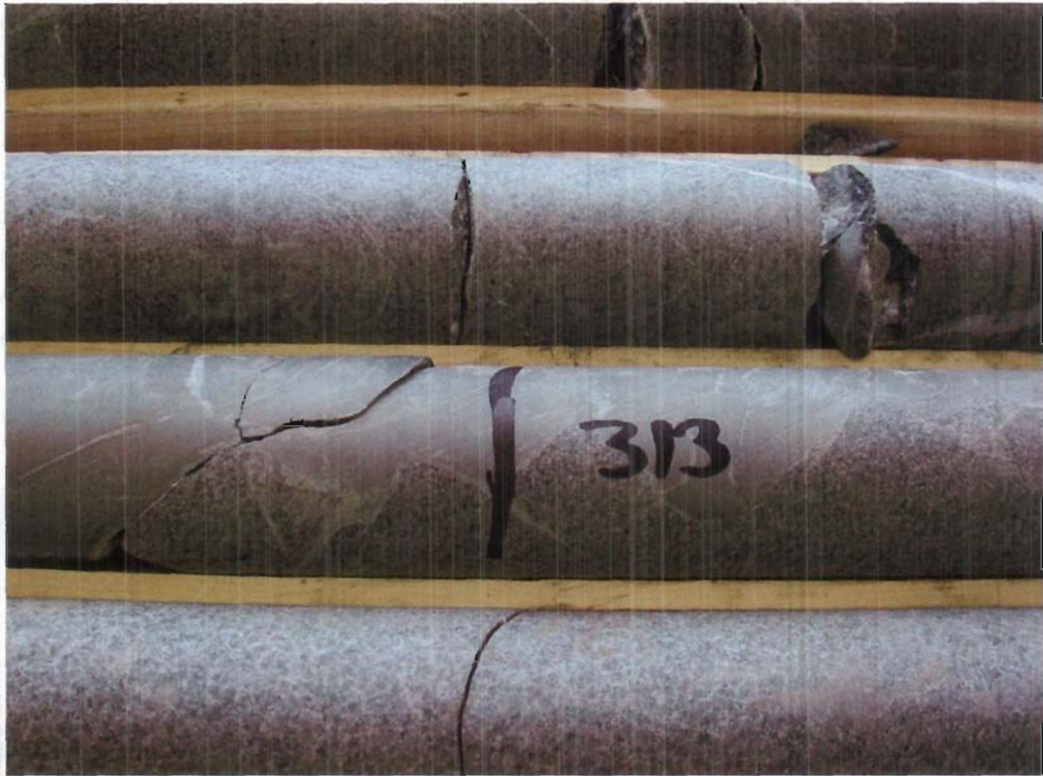
DSCN 2128. Late pulse 9T cutting coarser grained 9D melagabbro.
