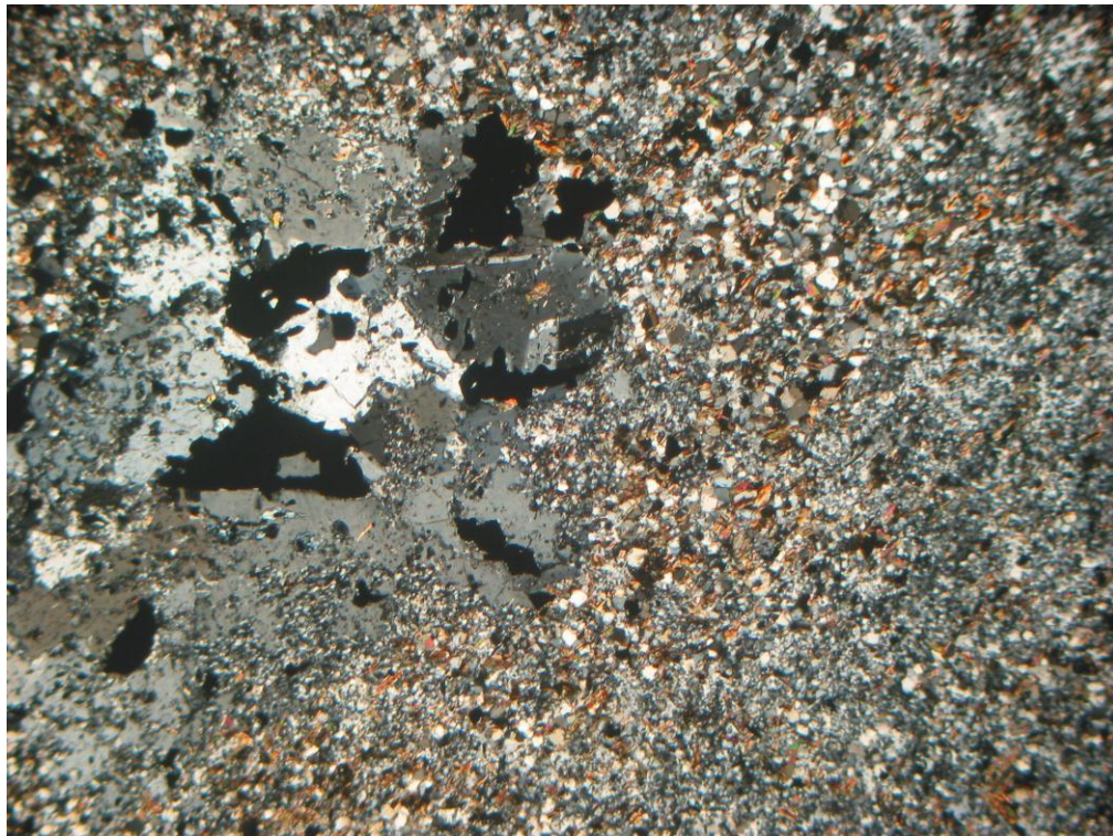
Heron Pond-4 Plate 1: Fine-grained biotite, Ca-plagioclase, and quartz matrix significantly without fabric, including a domain of coarsely crystalline Ca-plagioclase (An50) intergrown with pyrrhotite, a zone of ingress of hydrothermal solution.
