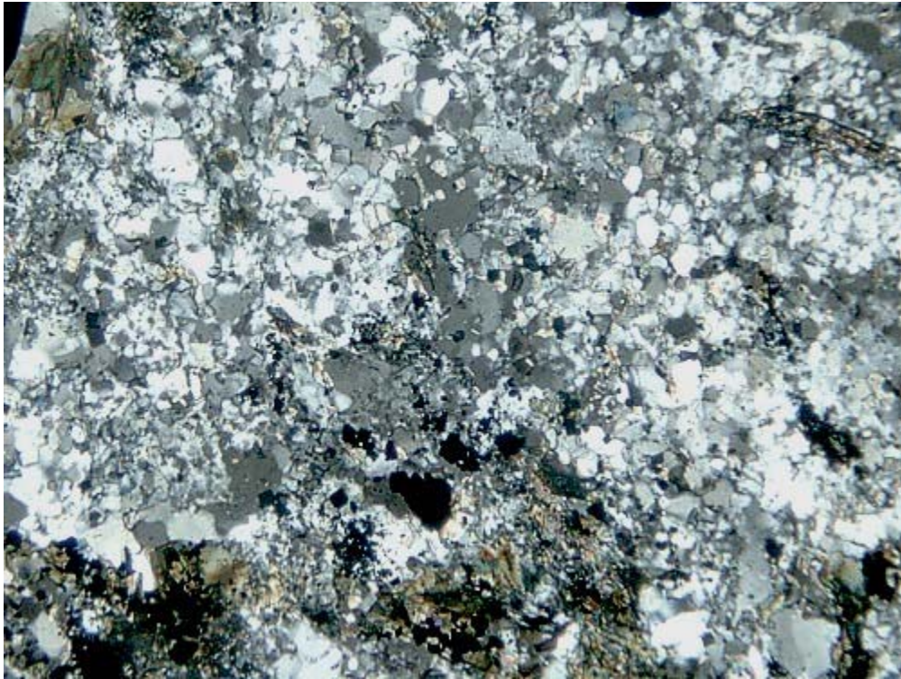
Granulated feldspars. X-axis of photo: 1.6mm. X.
