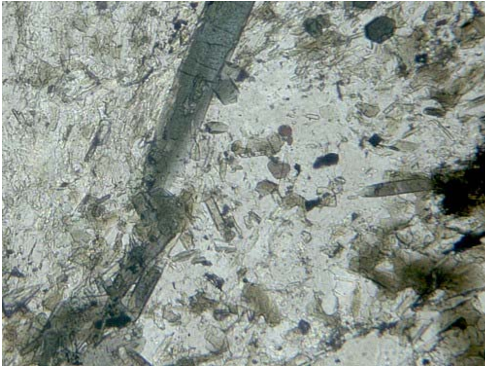
Long mottled green tourmaline prisms and small tourmaline grains. X-axis of photo: 1.6mm. Ppl.
