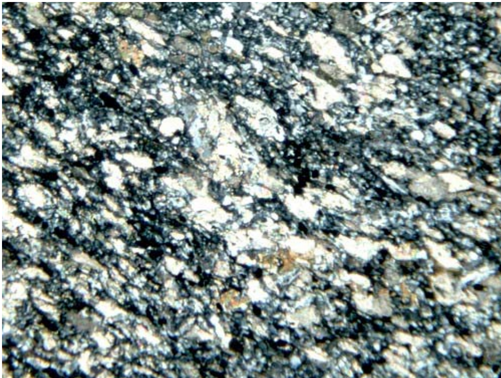
Carbonate (light grains) and interstitial green chlorite in andesite. X-axis of photo: 1.6mm. XN.
