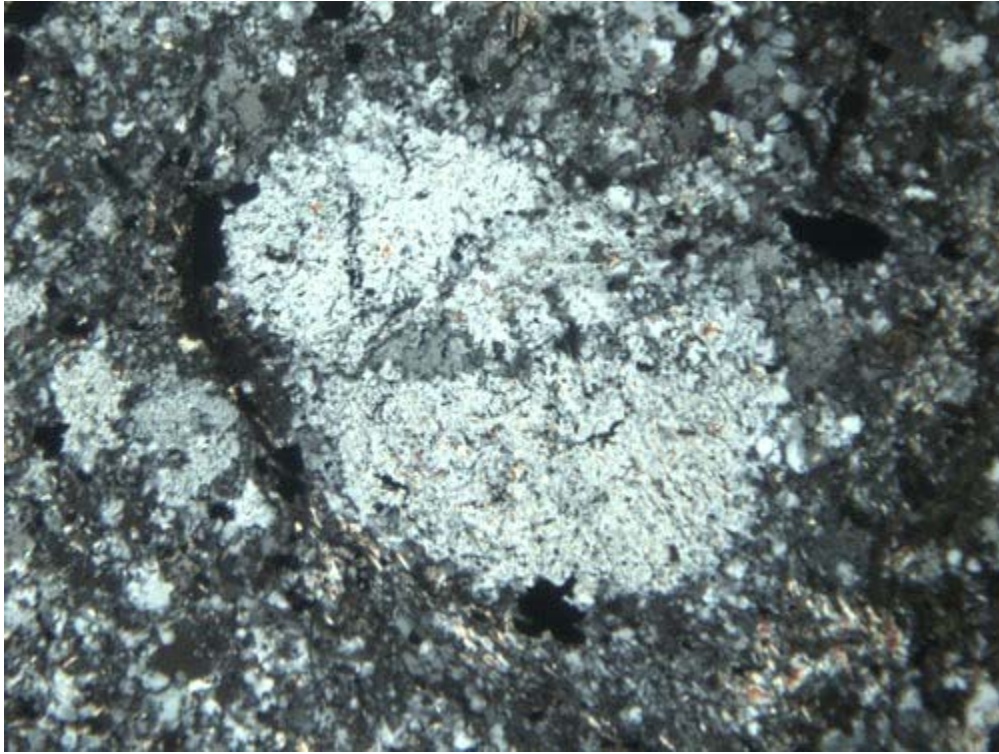
Relict, corroded plagioclase phenocryst. X-axis of photo: 1.6mm. XN..
