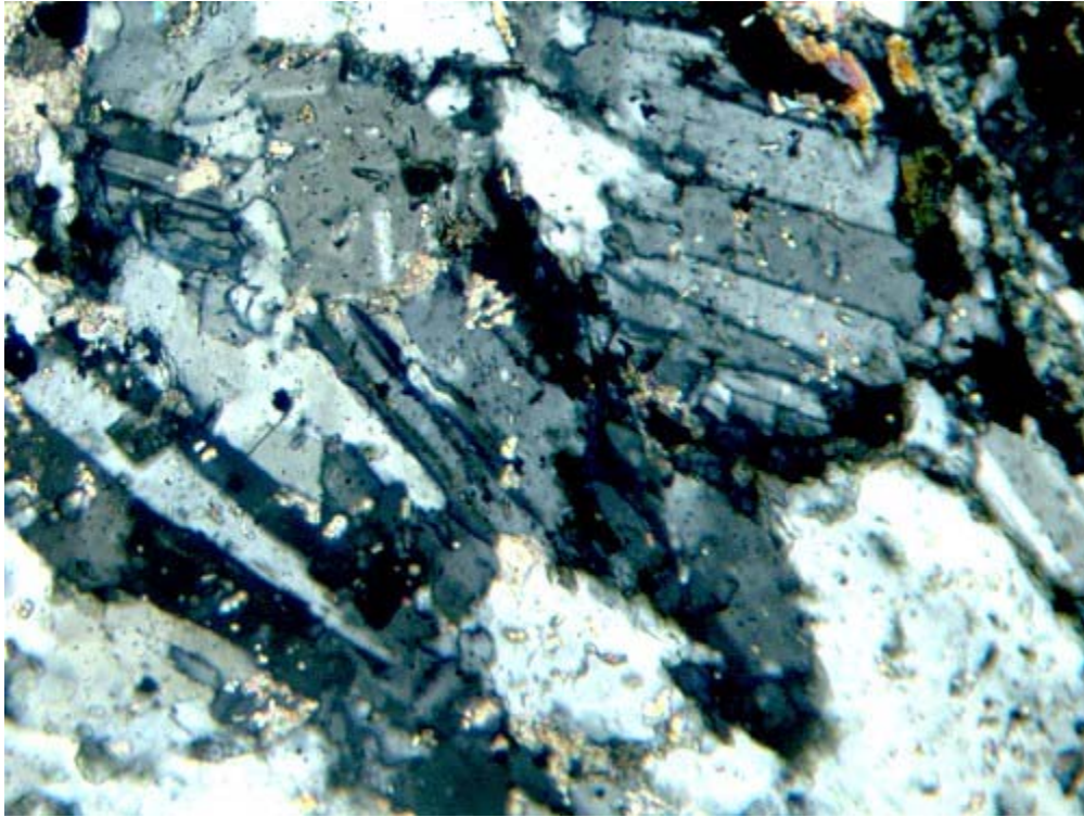
Secondary albite replaces original plagioclase (untwinned). X-axis of photo: 1.5mm. XN.
