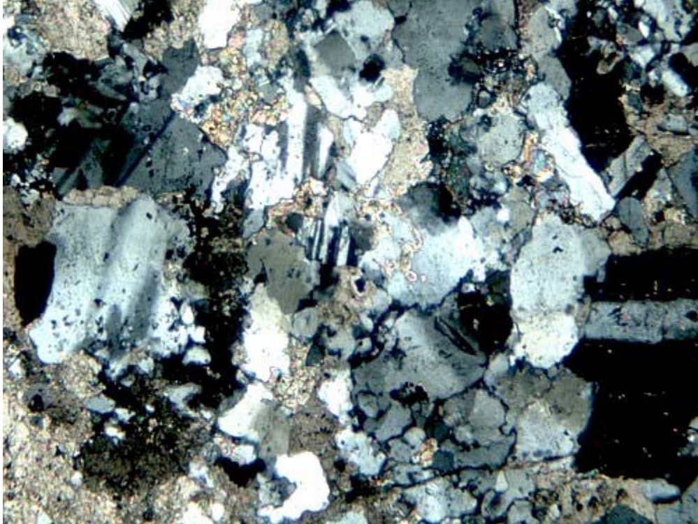
Relict plagioclase in carbonate-altered intrusive. X-axis of photo: 1.6mm. XN.
