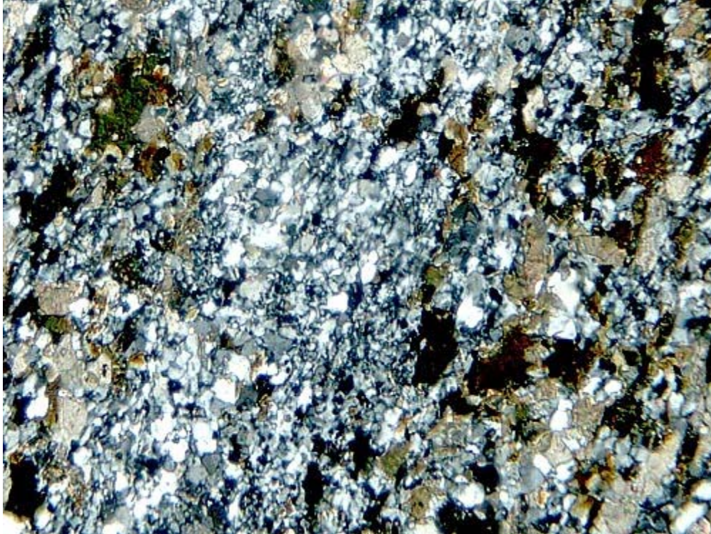
Fine-grained recrystallized and carbonate-altered rock. X-axis of photo: 1.6mm. XN.
