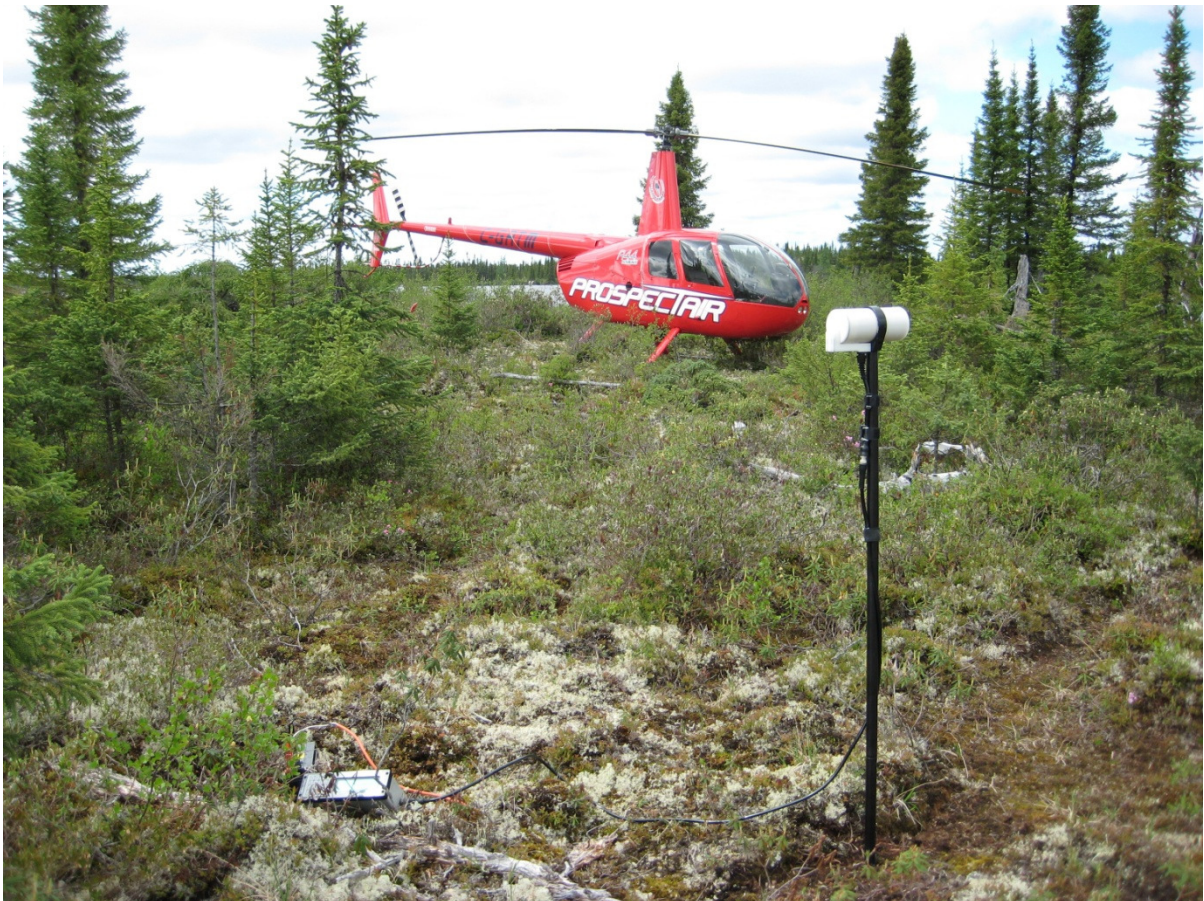
Figure 5: Magnetic base station setup at a fuel cache
