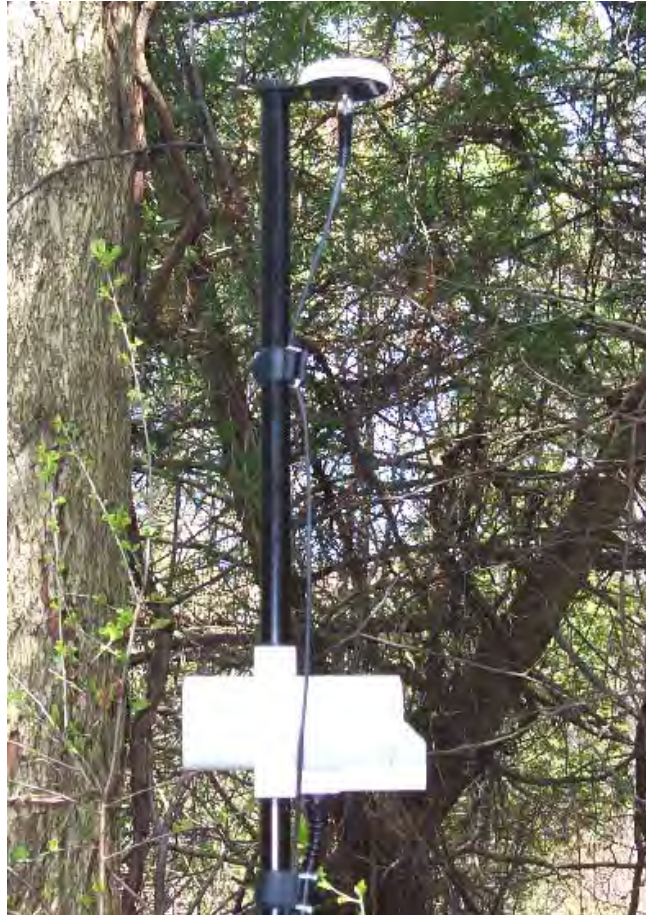
Figure 1: Sensor and GPS antenna. Use a full section staff (56cm) between sensor and antenna to avoid magnetic interference.
