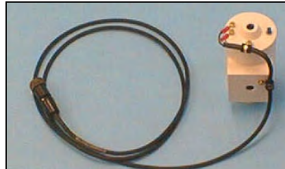
Figure 11. Top sensor with gradiometer cable attached.
