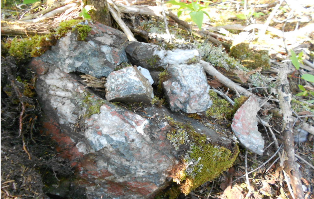
Figure 4 Hematite altered quartz-vein breccia in granodiorite from historical pit sampled by 744693 and 744694 returning low gold values of 0.006 and 0.010 g/t
