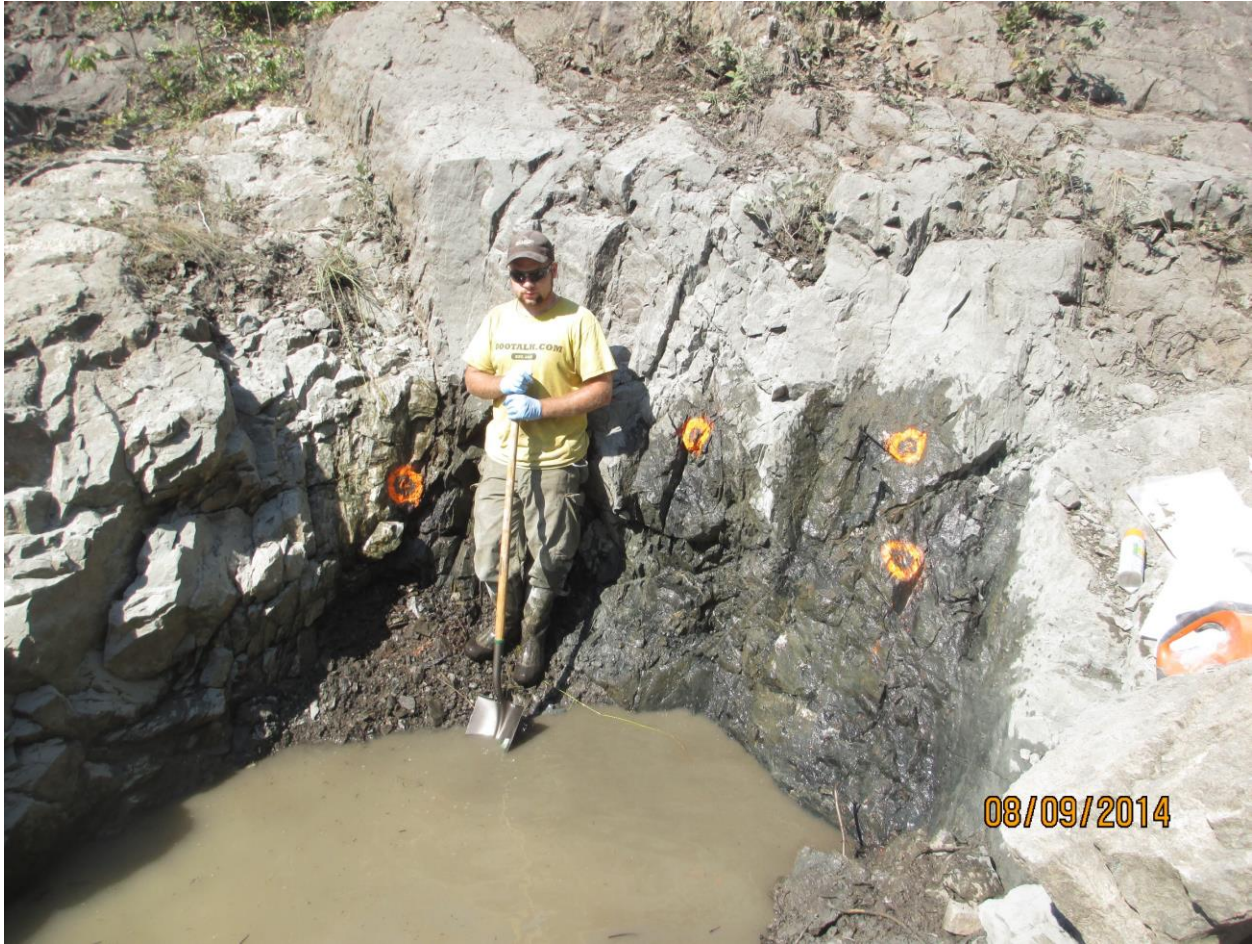
Photo 2 - Nixon-Bartleman shaft, looking northwest, showing locations of the four shaft samples taken (1409311-4).
