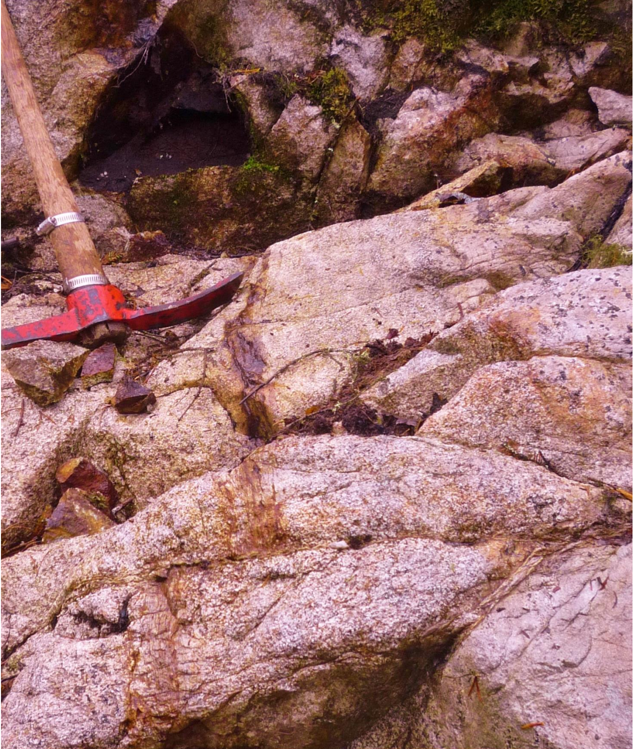
Figure 10. Nickel-copper bearing sulphide veins in gabbro. 594742mE, 5366472mN
