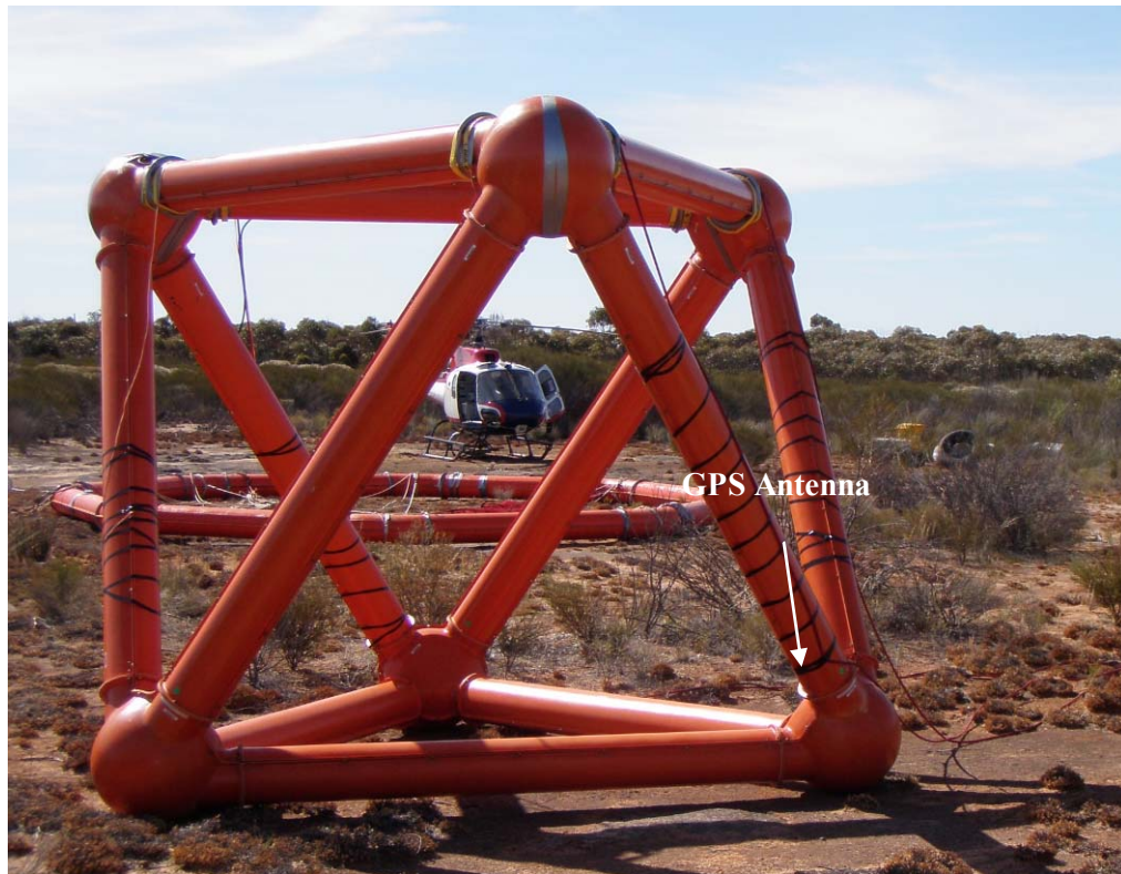
Figure 5: ZTEM base station receiver coils.
