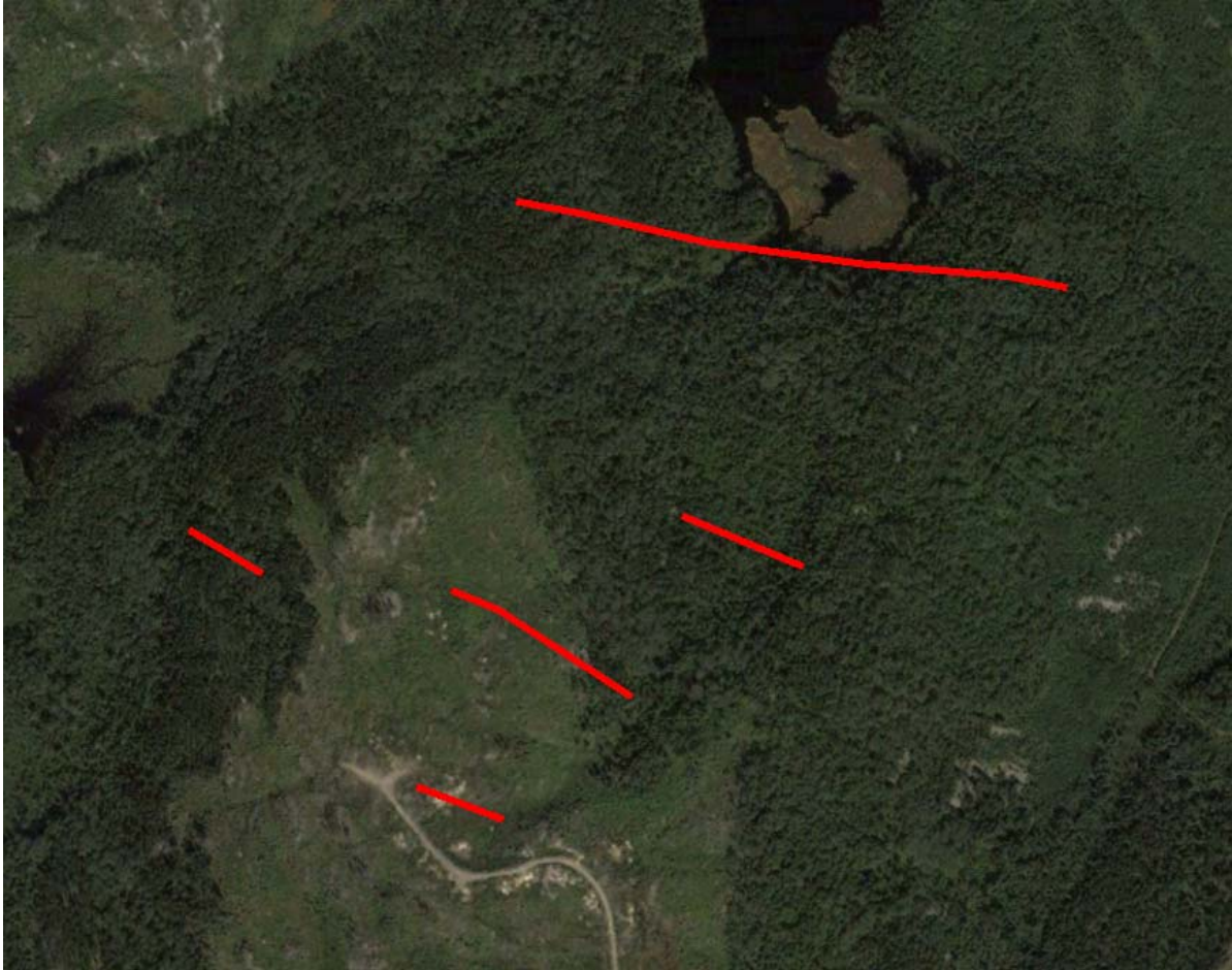
Figure 3: Google Image with the VLF EM Axis Overlays
