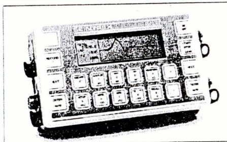
Front panel of ENVI-MAG showing a graphic profile of data and large-key keypad
