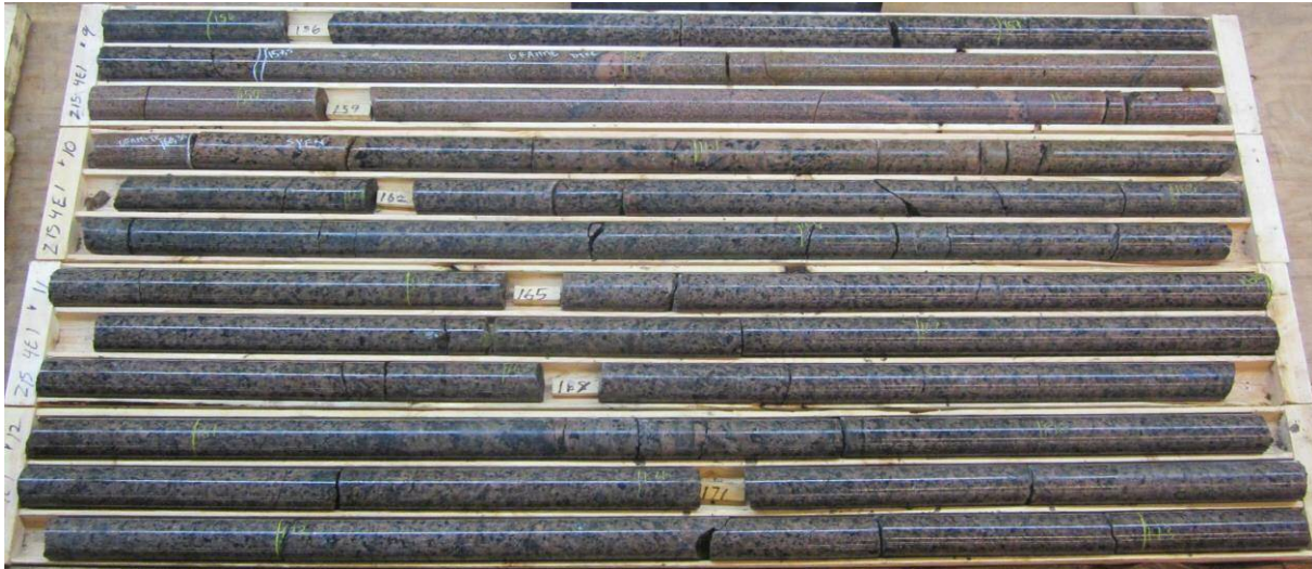
Figure 12: Typical medium- to coarse-grained amphibole syenite with pink granitic dike from approximately 156 m to 173 m.
