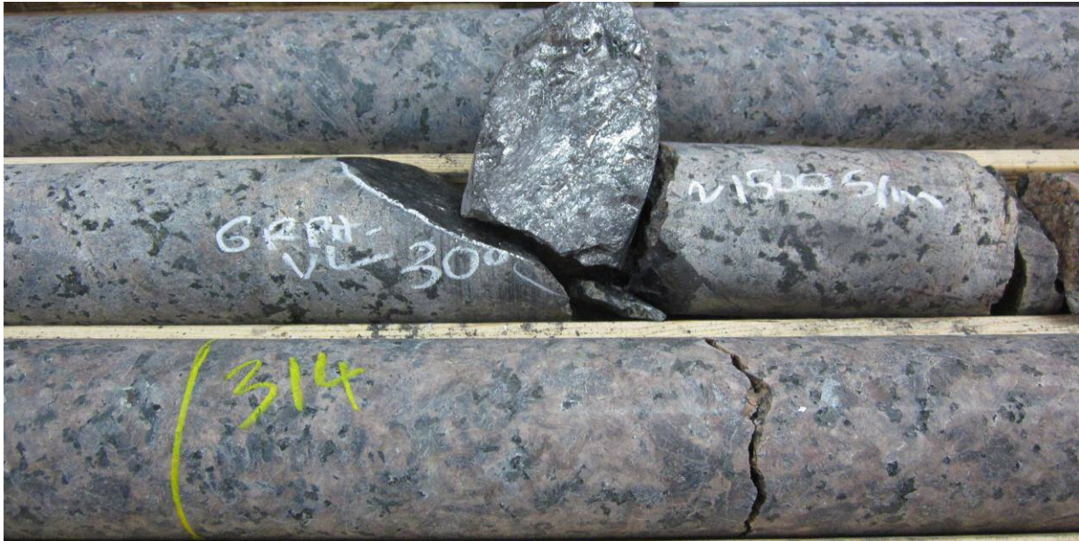
Figure 14: Graphite-filled hairline veinlet at 312.75 m in syenite
