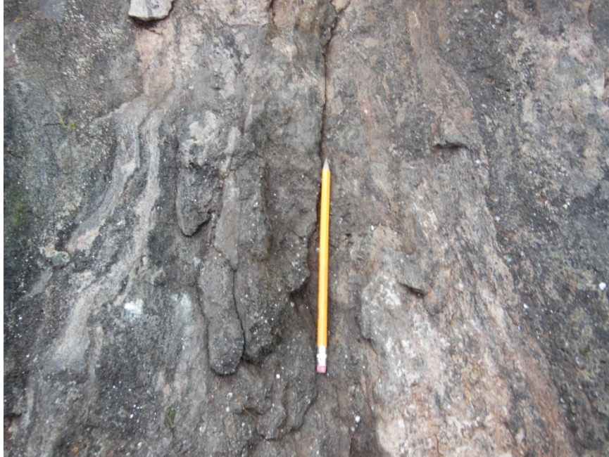
Photo 15. Strongly radioactive gneissic felsic rock with glimmerite pod marked by pencil in large angular boulder near cliff at Pole Lake REE-Nb-Th-Ba showing.
