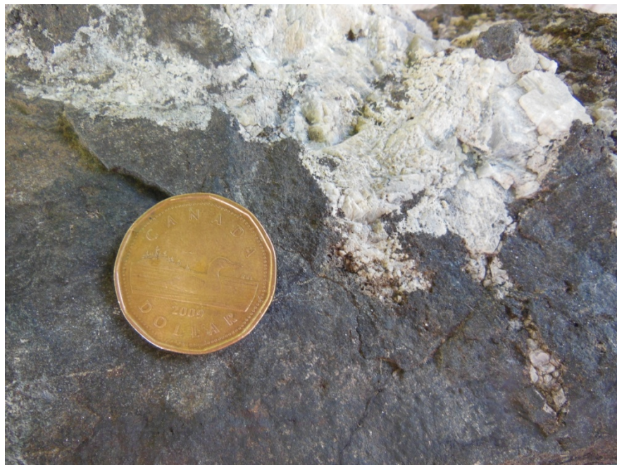
Photo 10: Magnetite-rich rock from old test pit that shows gradation into calcio-carbonatite segregations.
