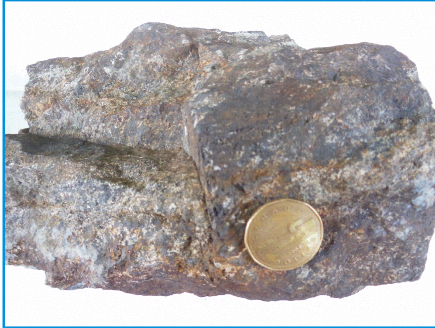
Photo 13. Large piece of subtly layered, magnetite-rich material from old pits near Camp Lake Road at UTM 340773E, 5294697N. Dark brown area is rich in magnetite and disseminated white fine- to medium-grained minerals may consist of REE phases, barite and nepheline. Spectrometer measurement on sample: 2.0 %K, 0.0 ppm U and 383.3 ppm Th.
