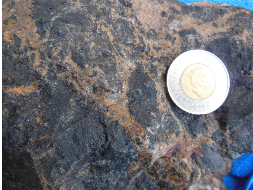
Photo 6. Abundant orange mineral that occupies the interstices of magnetite-rich rock from boulder near largest test pit on Beaver Pond. Spectrometer measurement on large block: 2.7%K, 74.4 ppm U and 359.2 Th.
