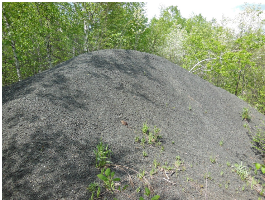
Photo 4. Pile of magnetite-rich concentrate situated near test pit at Zone 6 apatite-magnetite deposit, former Multi-Minerals property near test pits on Beaver Pond.
