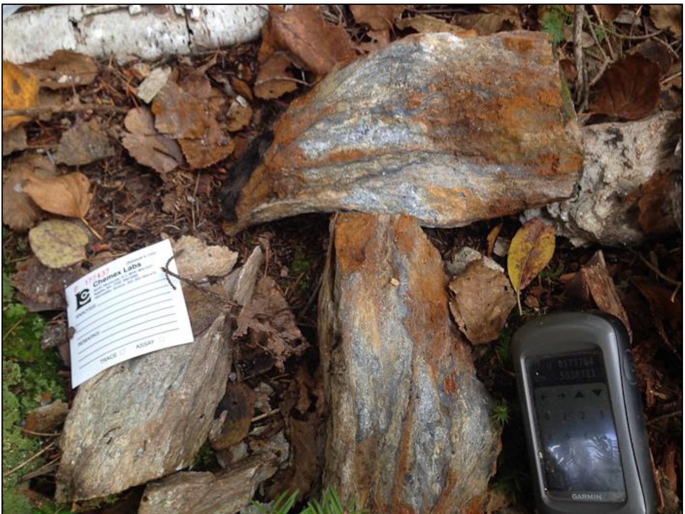
Photo: Sample 177437 from historical trench sub-crop of a quartz-carb vein which assayed 220.00 g/t Au
