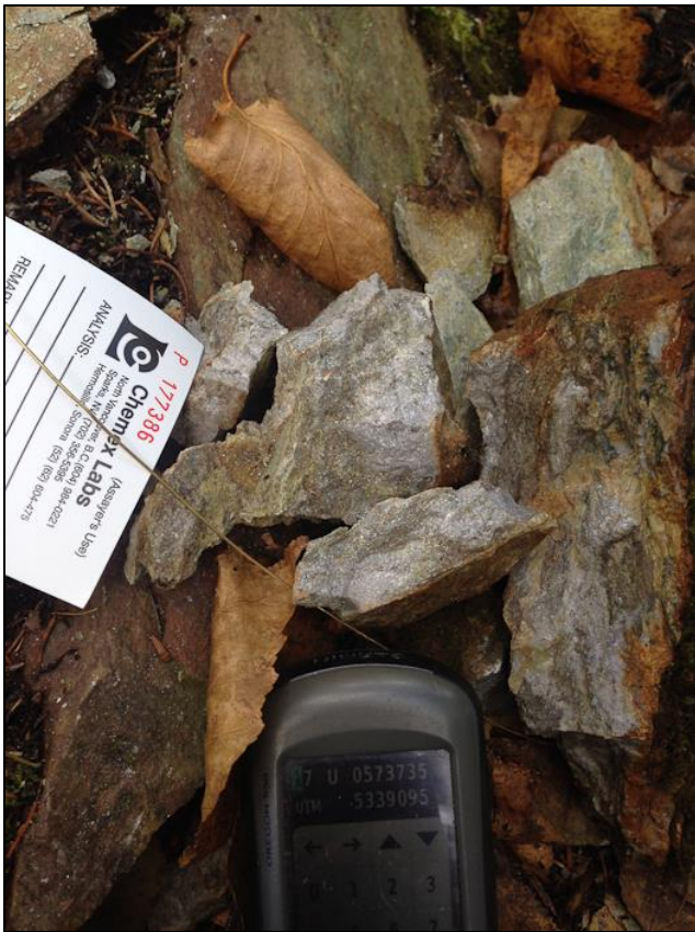
Photos: Sample 177386 which assayed 16.83 g/t Au (left), Sample 177337 which assayed 7.96 g/t Au (right)
