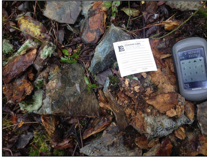
Photo: Sample 177411 which assayed 8.95 g/t Au taken from the shaft wallrock (above), Twin Shafts located along the Kirana Break where Sample 177411 was taken (below)
