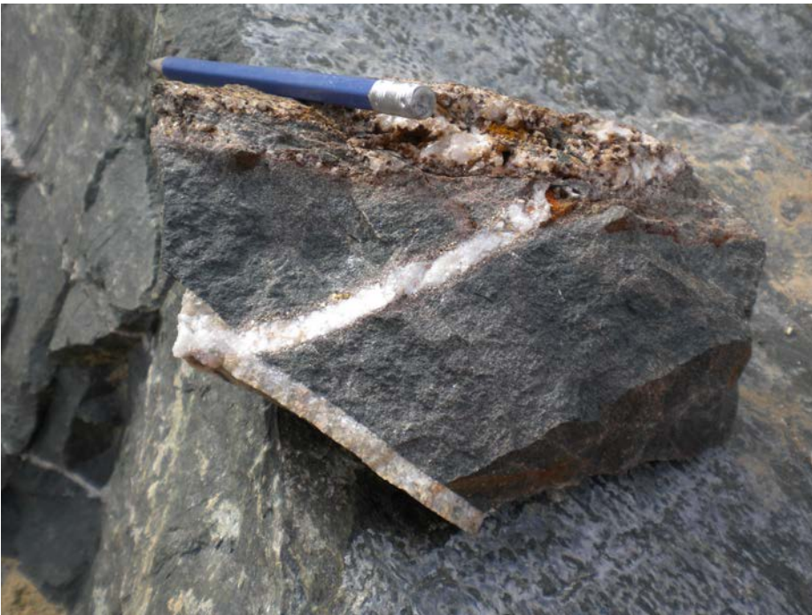
Photo 4 – Fine sulphide in narrow vein material.
