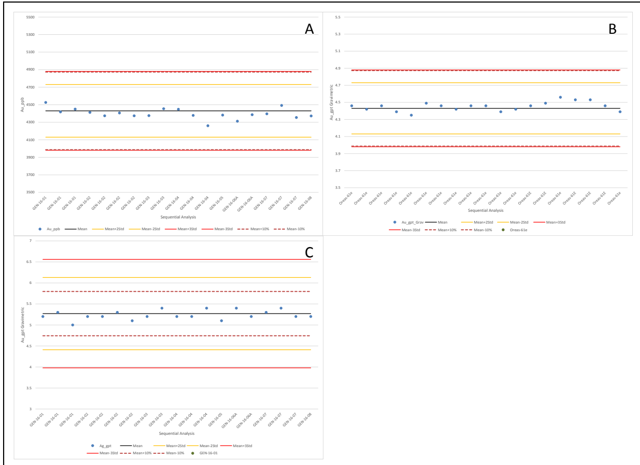
Figure 11: Control charts for Standard Oreas-61e for elements Au_ppb (A), Au_gpt_Gravimetric (B), and Ag_gpt (C).
