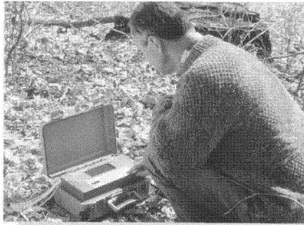
The IPR-12 Receiver measures eight dipoles simultaneously then records measured and calculated parameters in memory.
