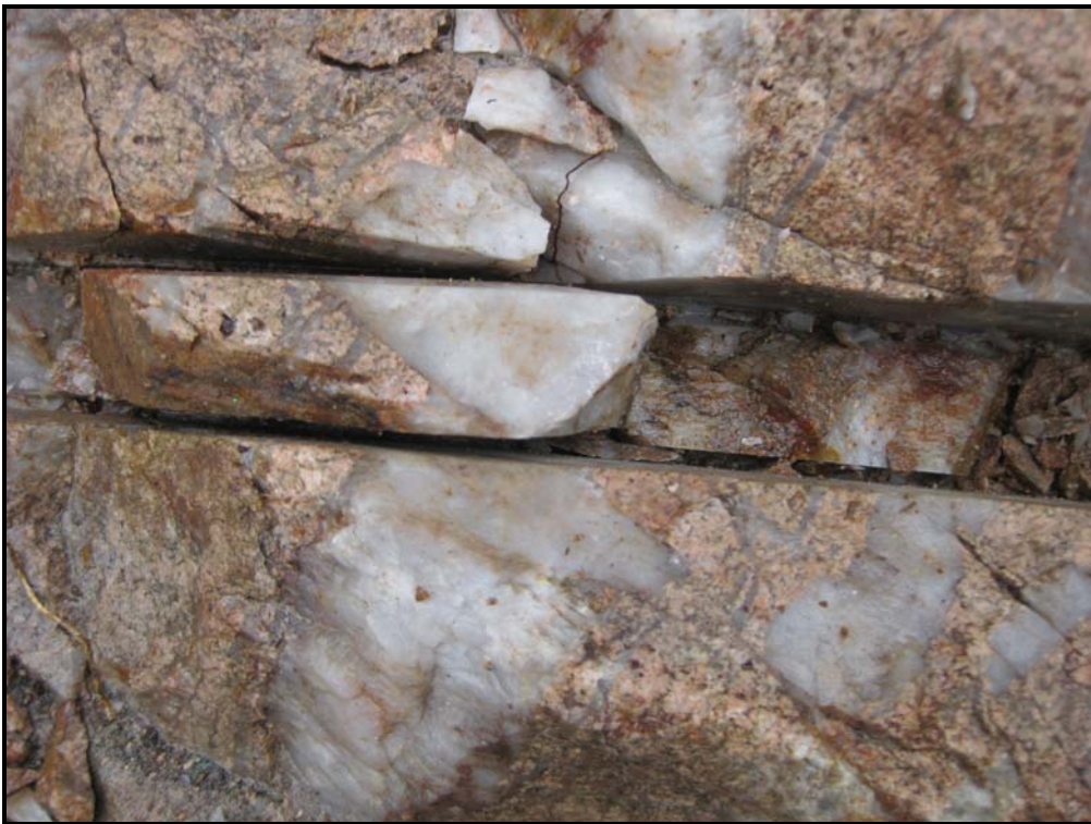
Top view of a late carbonate structure off-setting quartz vein @ 327-40
