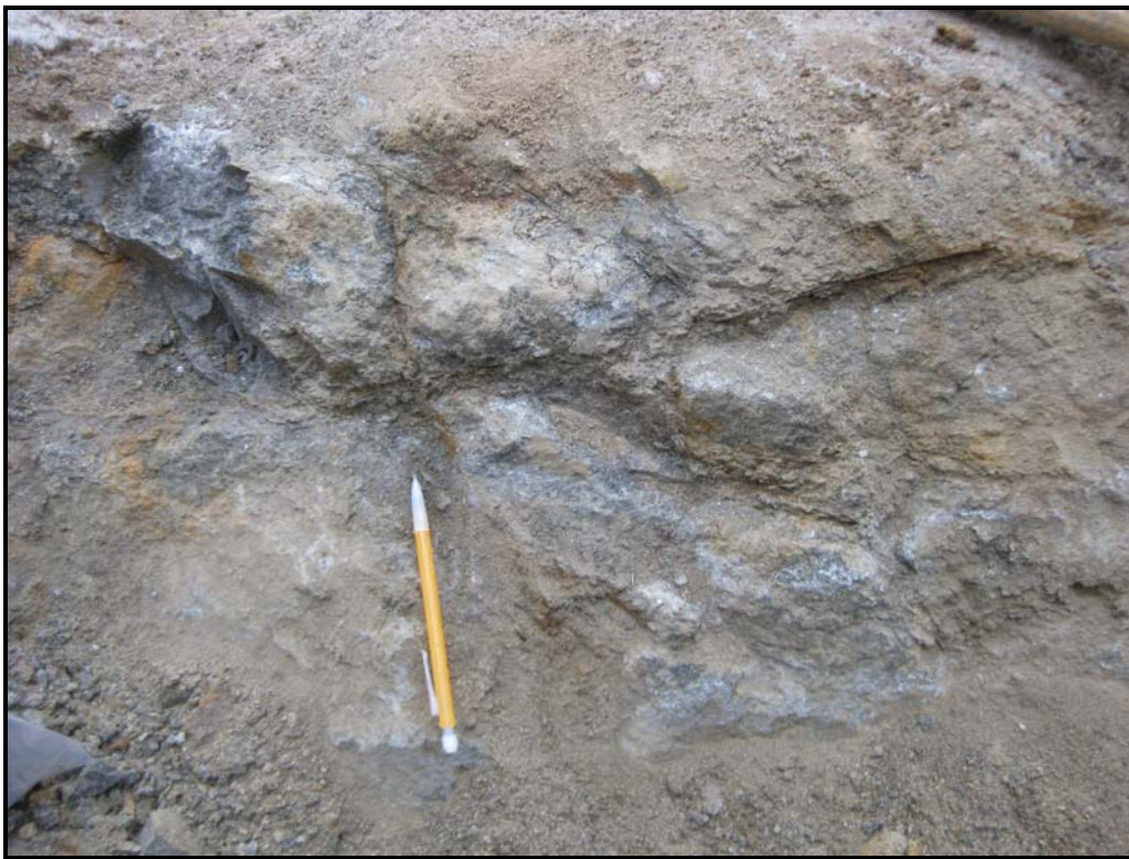
Well-developed fracture set at 312-85 cut by shallow north dipping shear (pencil pointing north)
