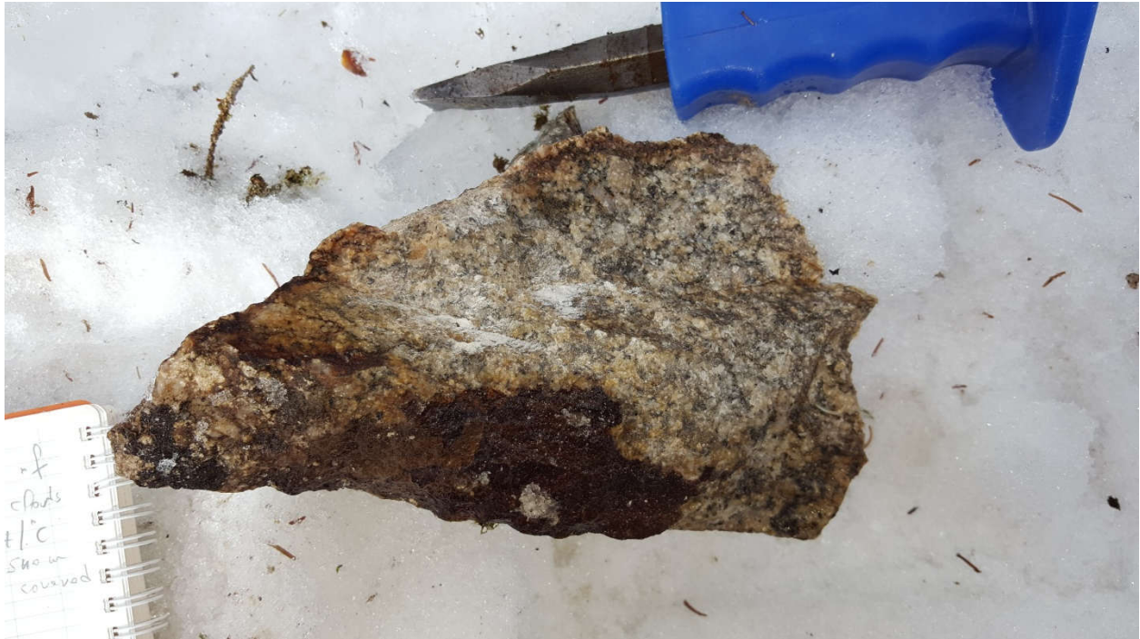
Close-up of sample FH17-01. Grey slightly pinkish coarse grained felsic intrusive rock.
