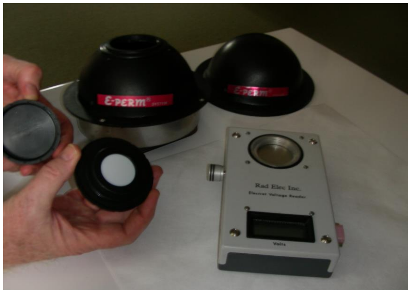
Principal components of the EIC System: At left electret with exposed white Teflon™ surface and cap; RFM with stainless steel collar; standard H Chamber; SPER-1 electret reader.
