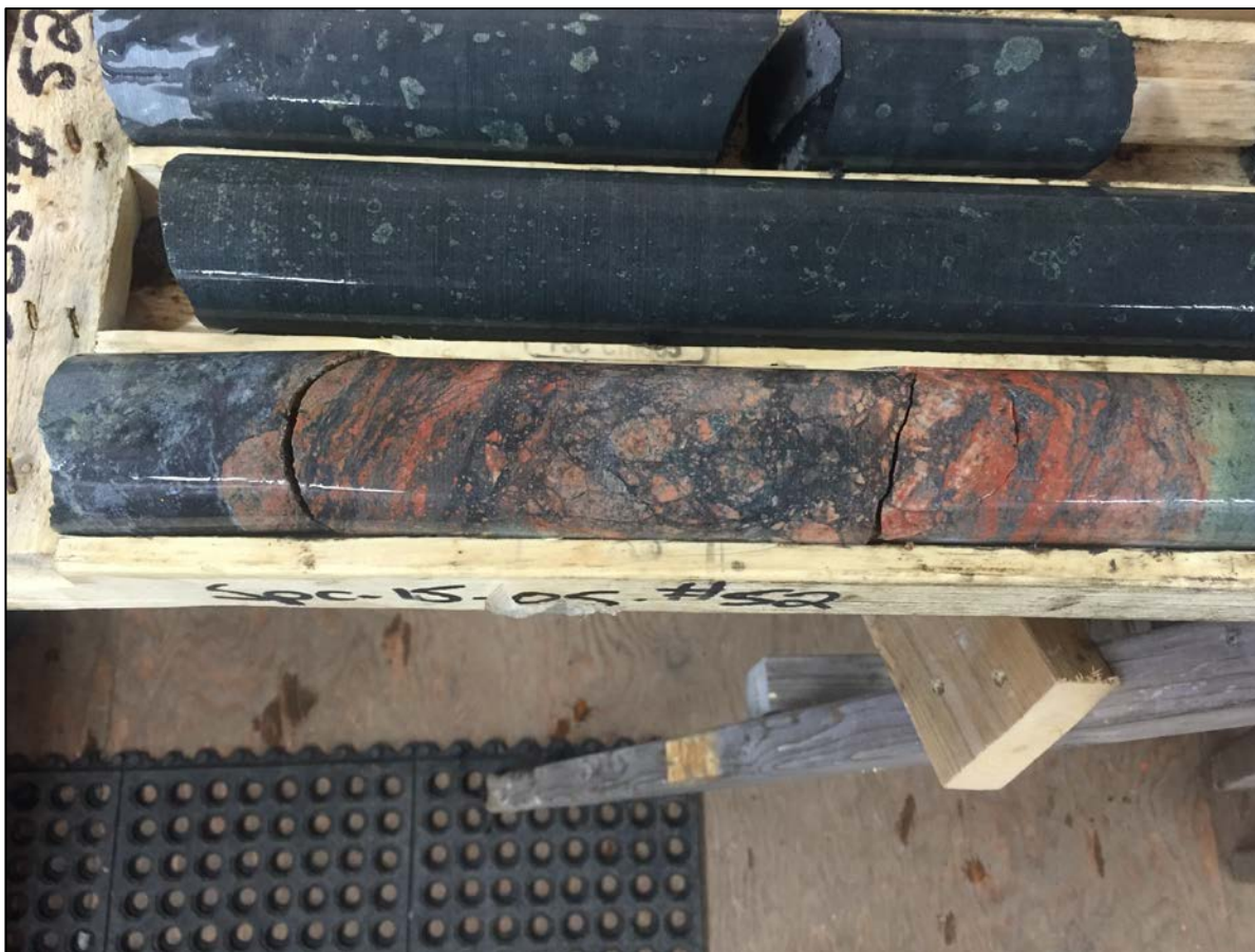
Figure 10 – A representative example of vein breccia with a magnetite rich matrix and strong epidote-potassic alteration of the wall rock.
