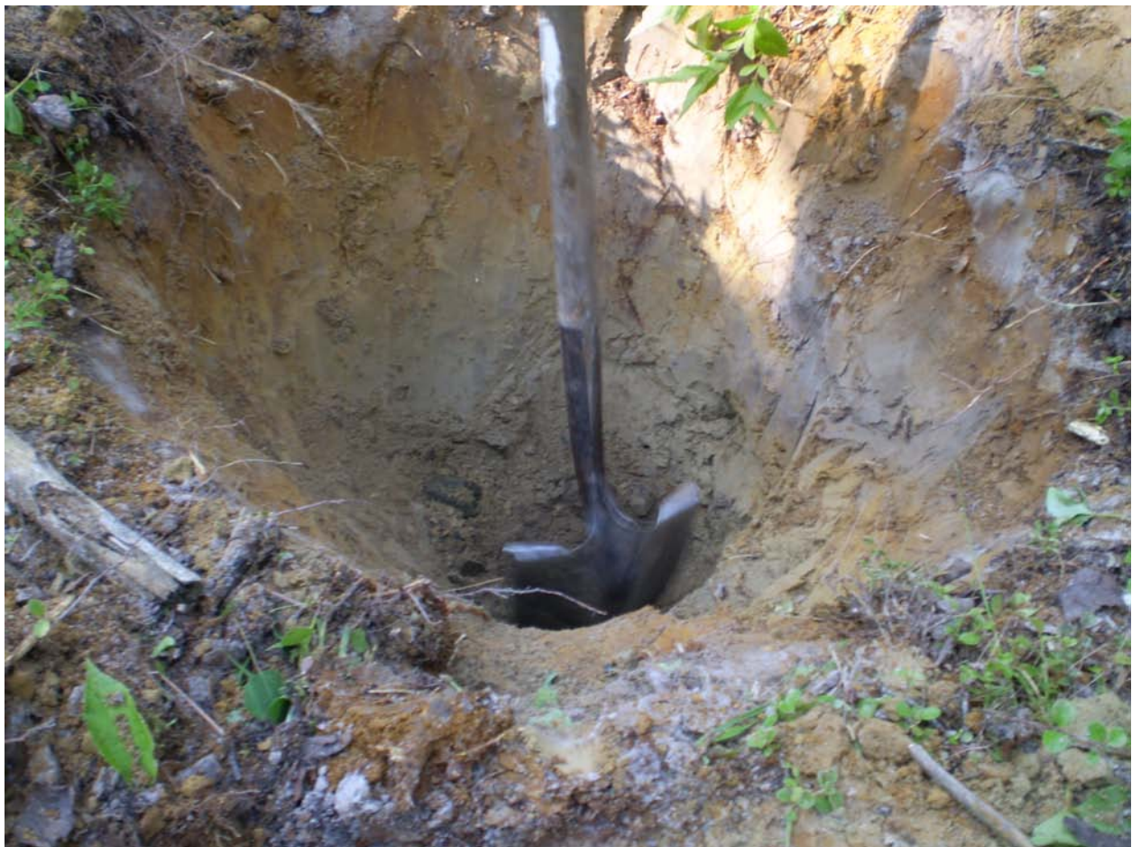
Figure 6 Photo sample site ML030 glacial till at approximately 1 m depth below 0.8 m thick layer of sand
