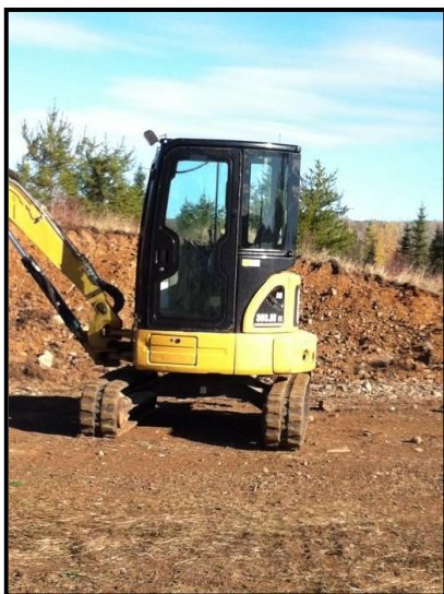
Photo 11: Excavator used for stripping
