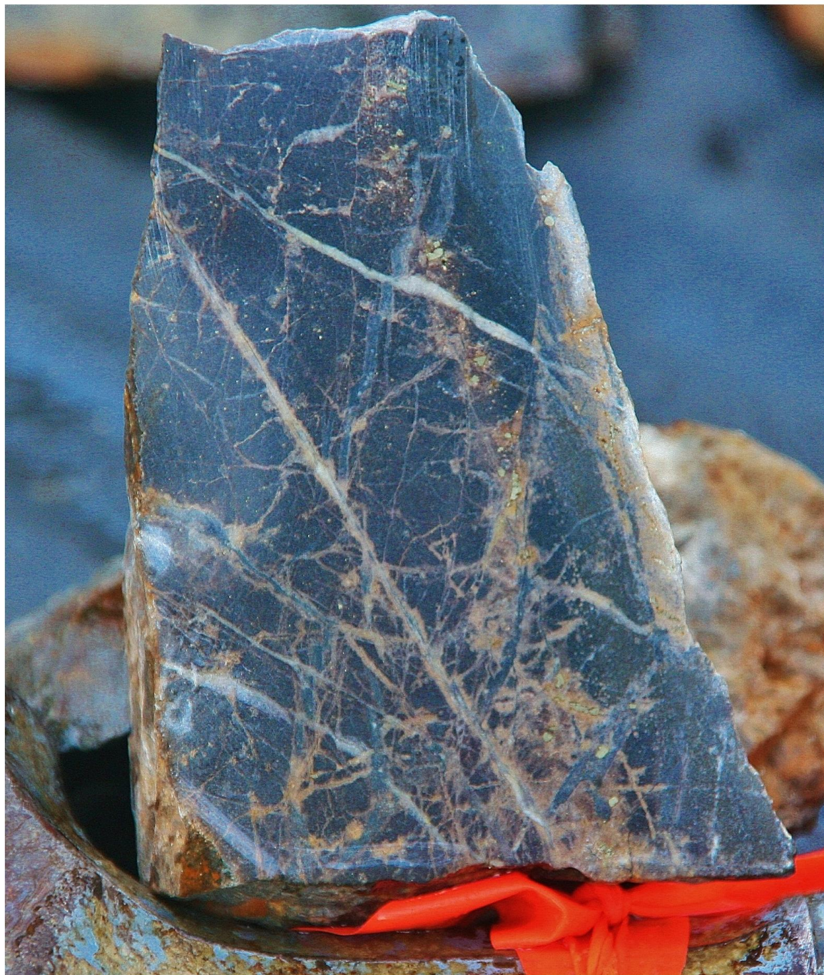
Figure 11. Central Trench: Pyrite, Hematite Stringers Multiple Generations of Quartz-Carbonate Stringers 4355937, Tannahill Twp. 594371mE, 5367030mN Brandy Brook Mines Limited
