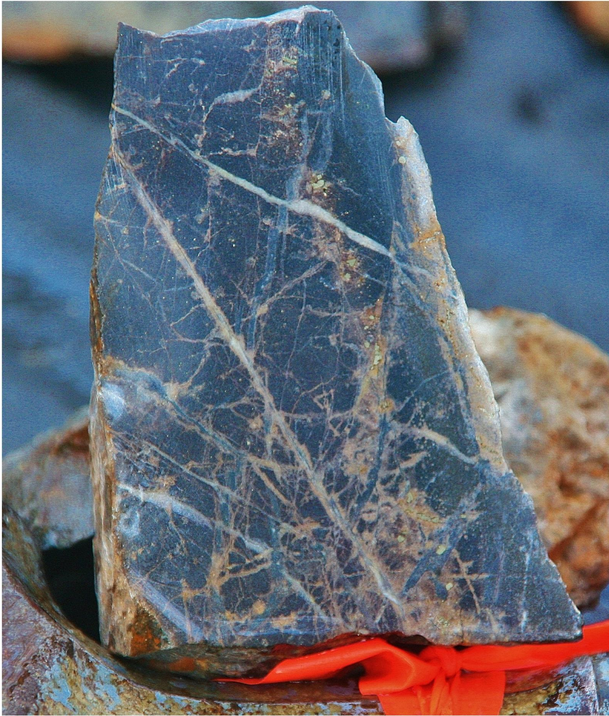
Figure 5. Fractured basalt with calcite-ankerite-quartz fracture filling, pyrite and hematite.
