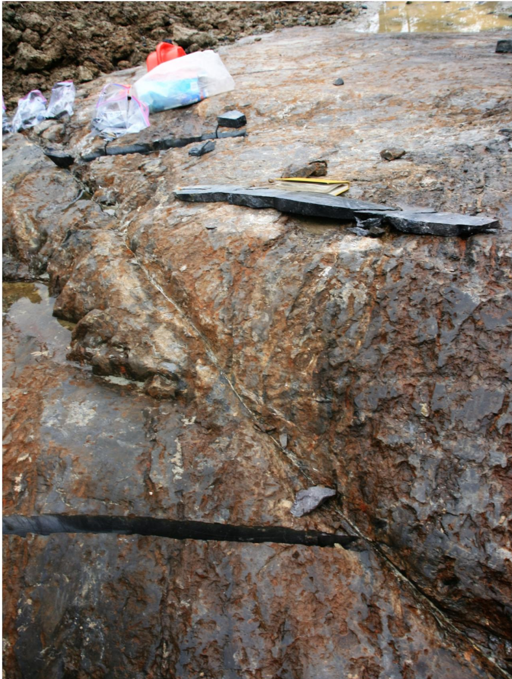
Figure 11. Fracture striking 48^{\circ} through Cut D and Cut A. Note thin quartz vein in fracture. Looking west
