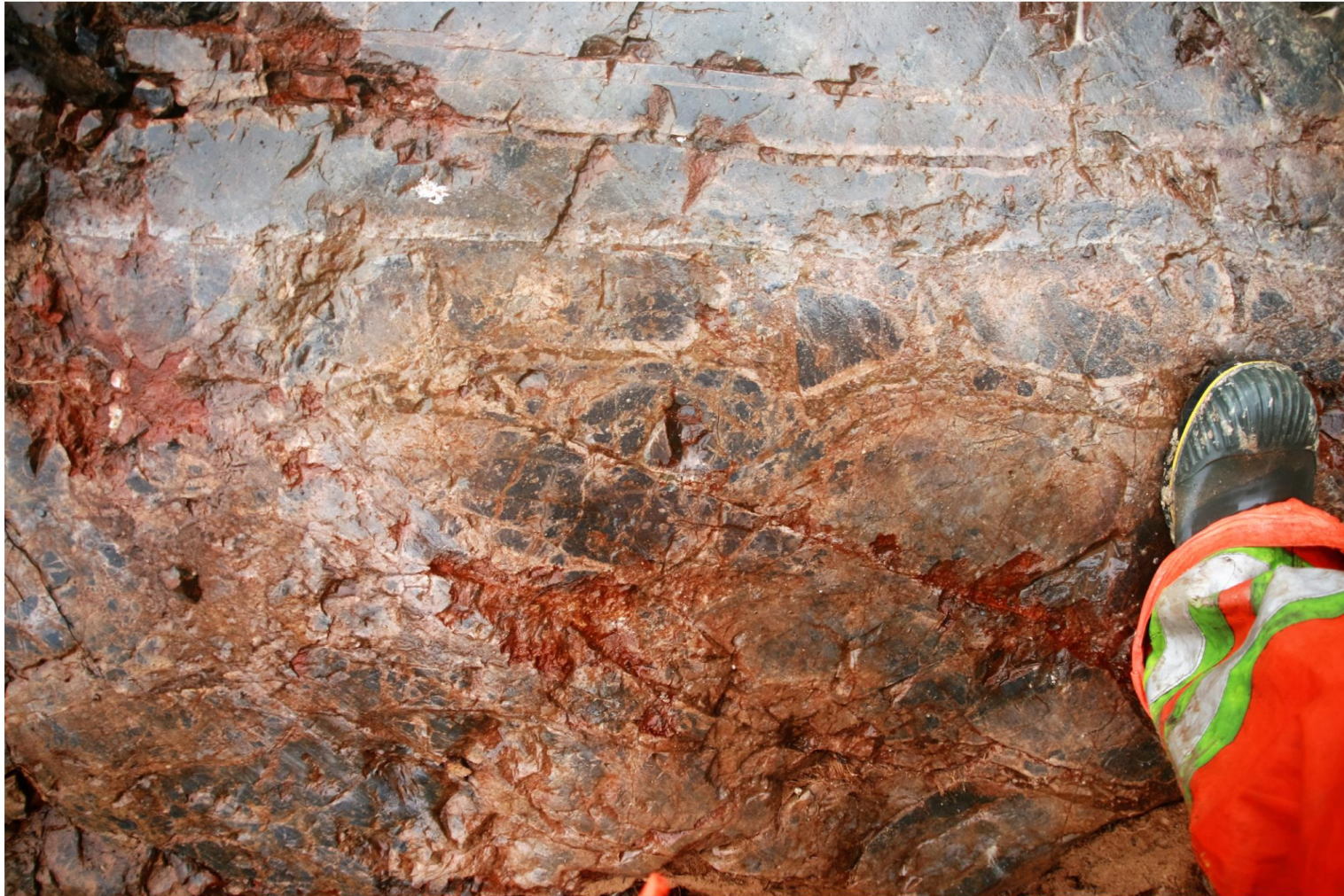
Figure 9. Breccia with carboante alteration and carbonate stringers. Looking south.
