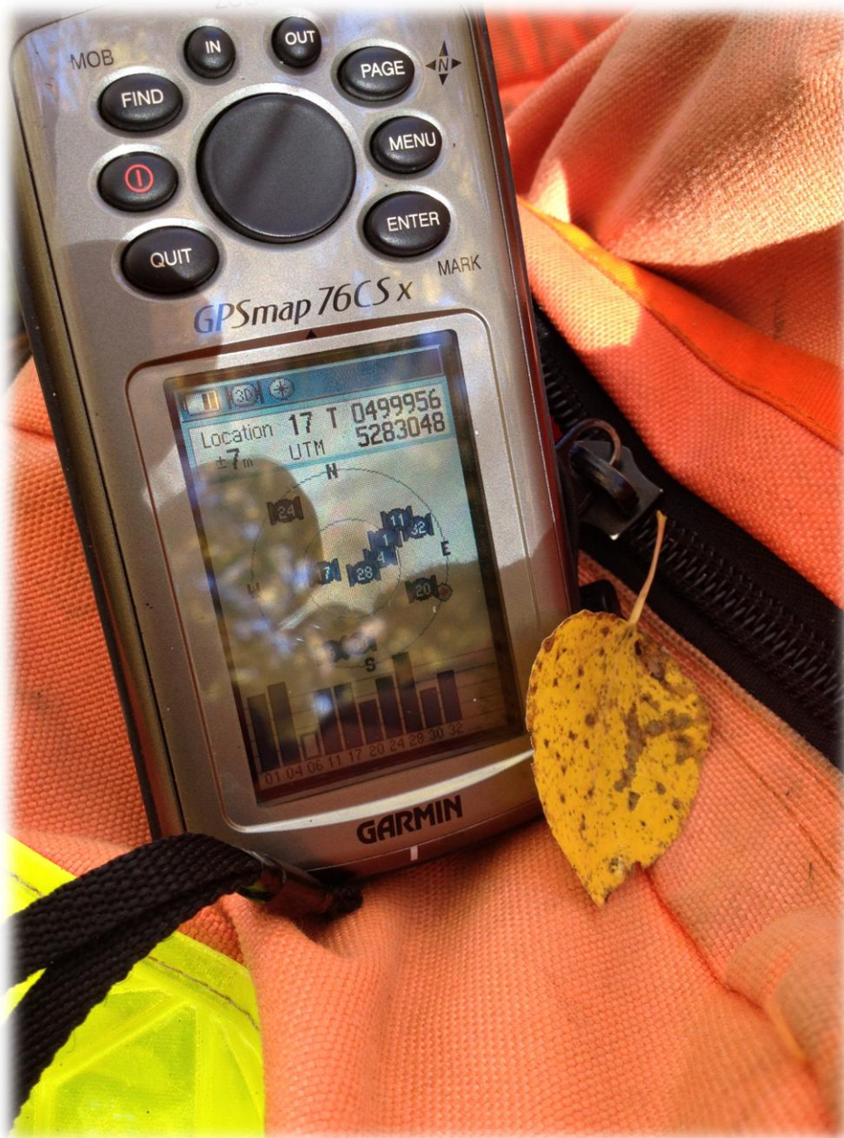
Photo of GPS showing location was taken at each sample station.
