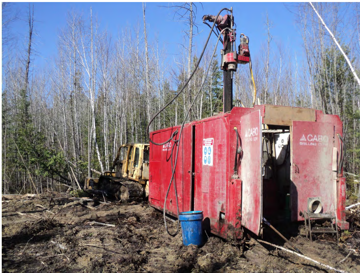
Figure 5 Skid mounted reverse circulation drill rig, Cameron 2012
