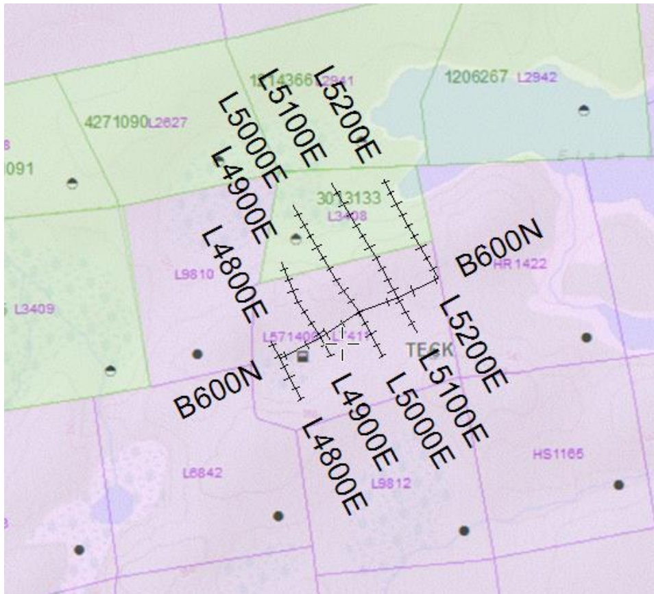
Figure 2: Cut Grid Sketch on Claim Map
