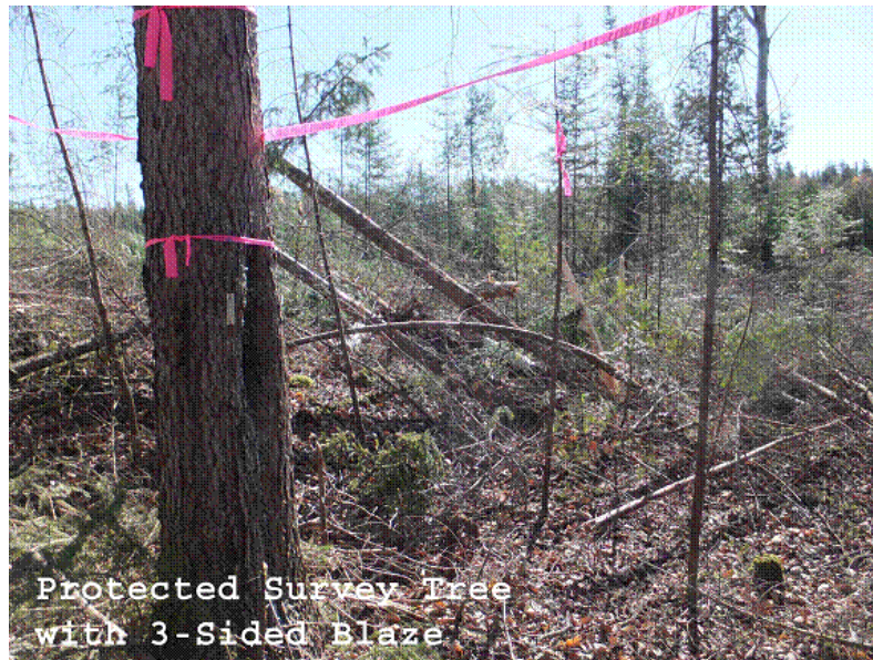
Photograph of Solitary Protected Surveyor Tree with 3-Sided Blaze Neighbors Claim Posts above
