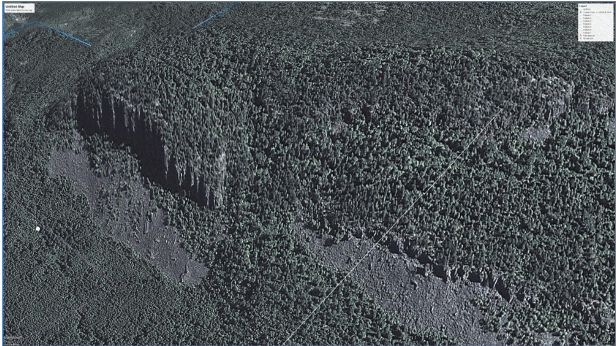
Figure 16: Fault zone defined by the difference in the diabase sill on either side of the fault. View to the northeast. There are two sills on the south side of the fault and one sill north of the fault. North is toward the upper left corner of the figure.
