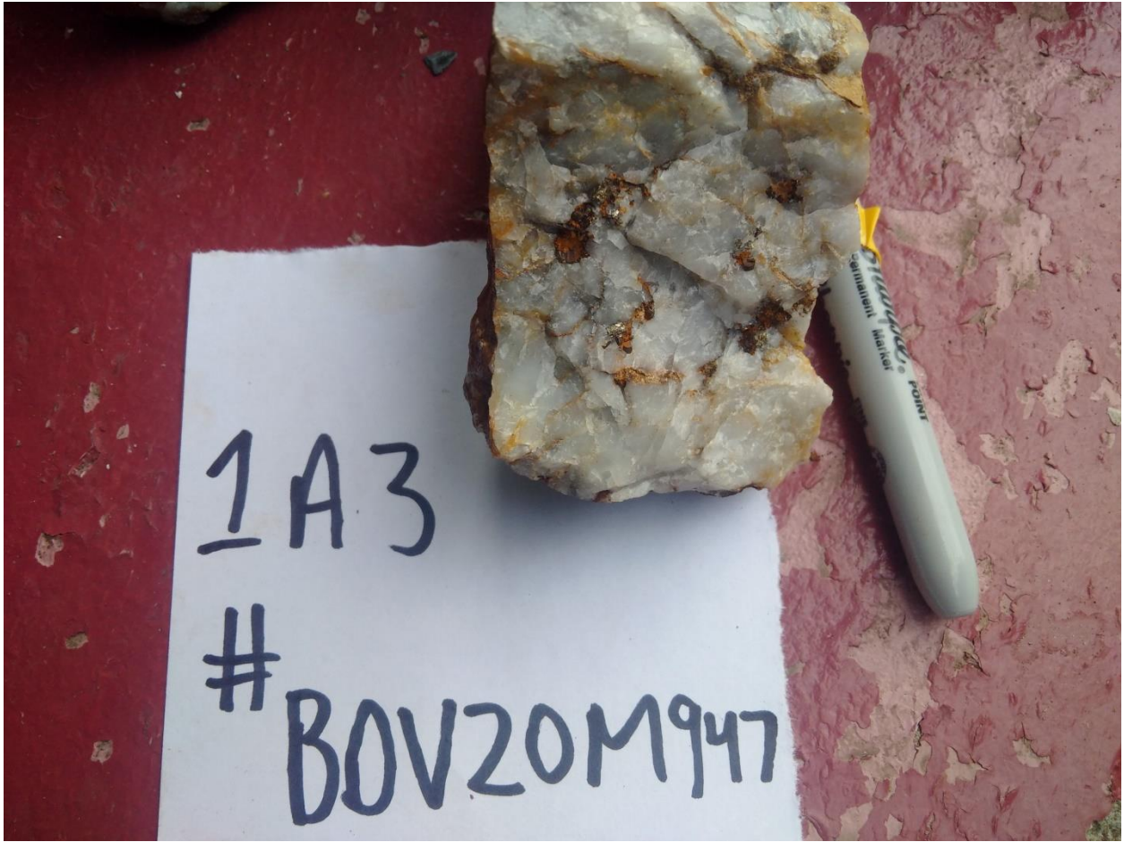
Figure 6. Highly fractured quartz with pyrite blebs. Assayed 4230 ppb au.
