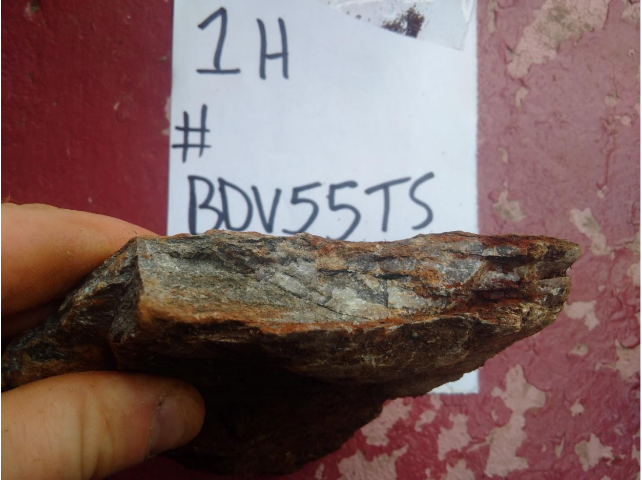
Figure 8. Highly sheared and mineralized mafic volcanic with small quartz veining. Assayed 384ppb au.
