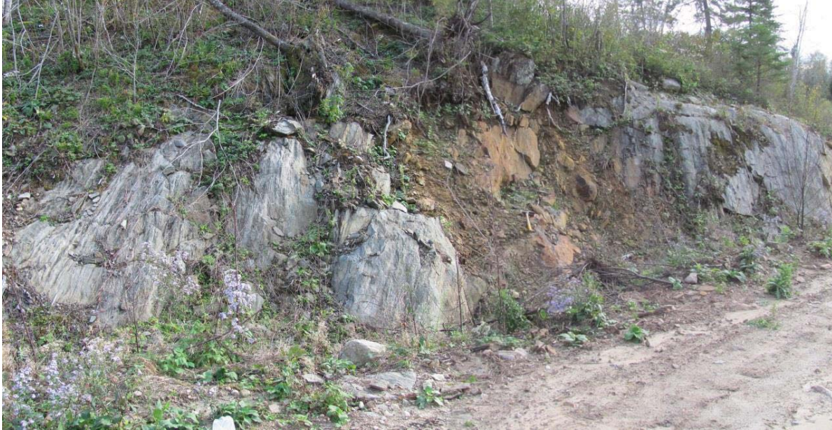
Figure 6: Stratabound iron oxide stained zone approximately 4m wide trending 005/85E-90 within greywacke sequence (Wpt 262 - UTM 449,872E 5,521,868N). The zone is weakly anomalous with respect to zinc and gold (437ppm Zn, 86ppb Au - ACA-003).
