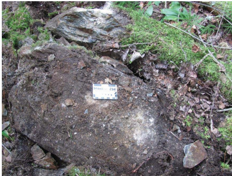
Figure 15: Minor topographic ledge on north facing slope south of Harrison Lake in close proximity to VTEM anomaly 6690A. Fe-oxidized siliceous metasediment/metavolcanic with 3-5% <1mm disseminated pyrite. Very angular float or possibly insitu. (Wpt 284 - UTM 451,297E 5,521,256N). Rock is weakly to moderately anomalous with respect to copper, lead, zinc and silver (156ppm Cu, 450ppm Pb, 920ppm Zn and 9.23ppm Ag - ACA-011)
