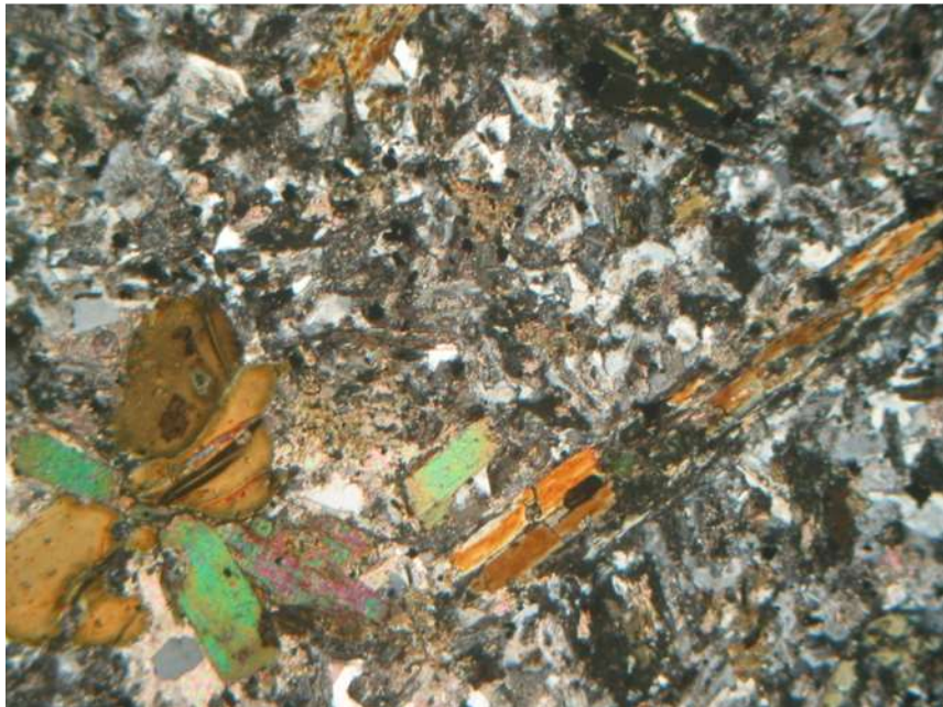
Radial cluster of biotite-phlogopite solid solution and lath shaped amphibole phenocrysts in a matrix dominated by finer-grained, randomly oriented plagioclase feldspar.
