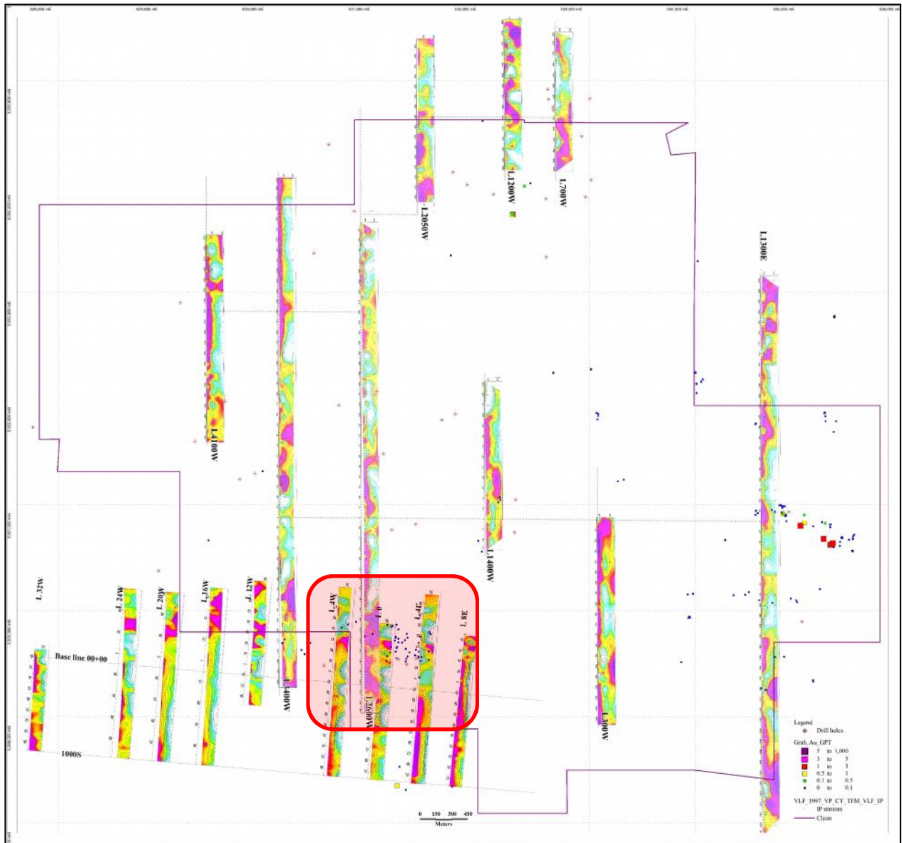
Figure 3. 2D IP inversion sections from 1997 survey plotted in plan view with overlap from current survey outlined (red box)
