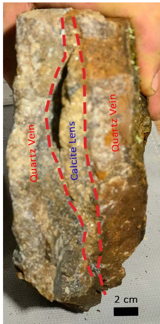
Figure 15 Sample ID K934654 from Black Jack North showing a carbonate lens with vuggy contact bound by quartz vein material.
