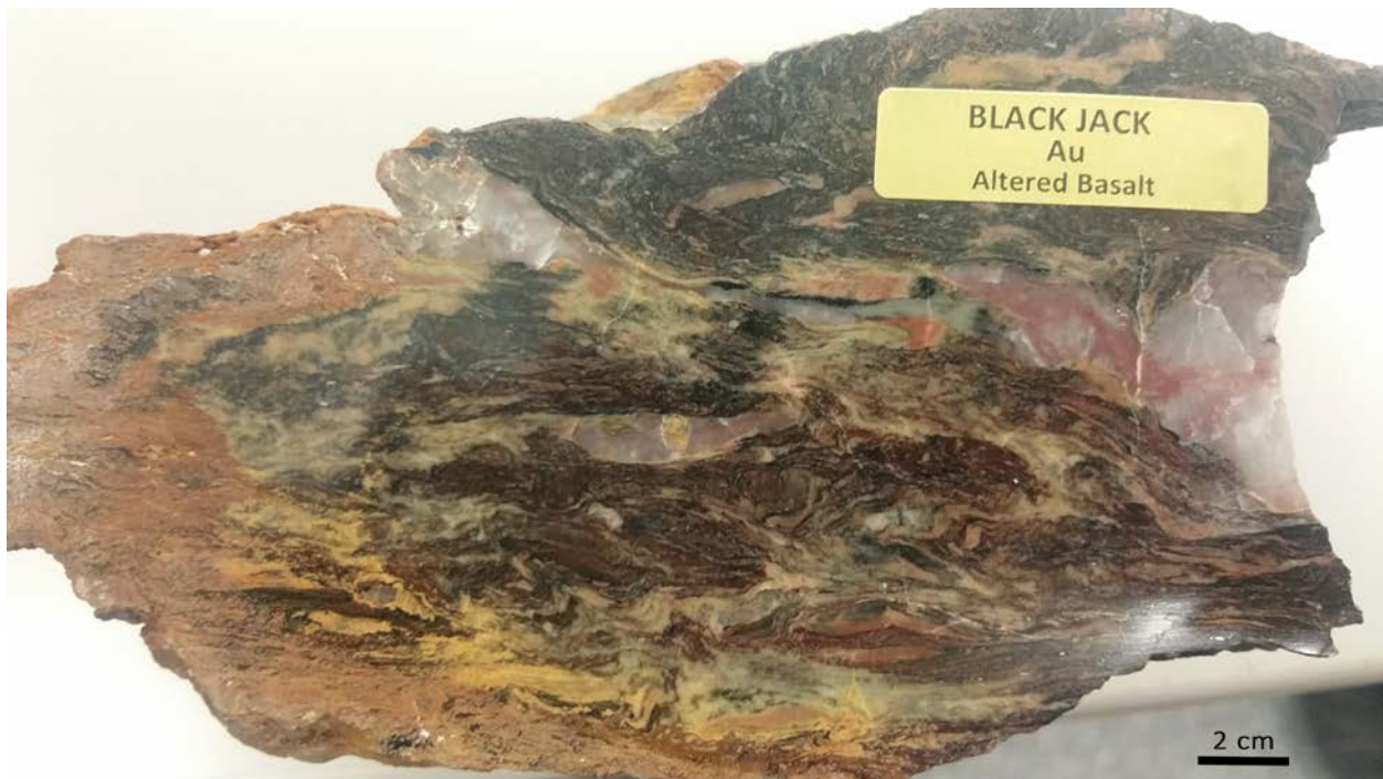
Figure 14 Picture of sample at the Ontario Geologic Survey's Kenora office of a cut and polished sample taken from the Black Jack shaft area of quartz veining in altered basalt.
