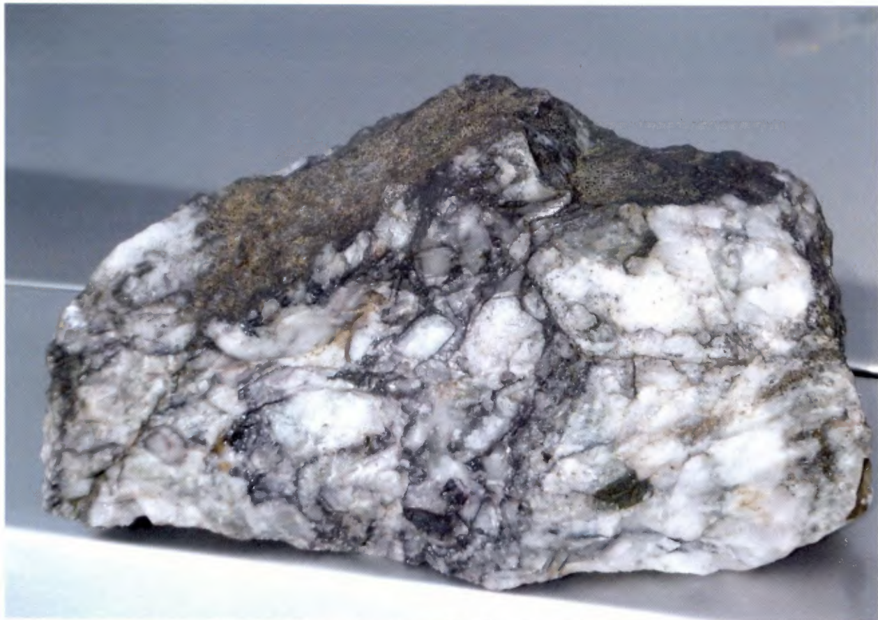
Photo 4: Specular Hematite filled quartz breccia.
